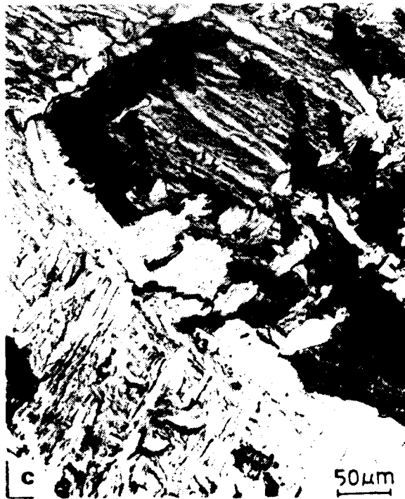
Figure 5 Optical micrographs of beta solutioned (2280°F) and annealed (1141°F) Ti 3 Al alloy. Kroll's etchant.
