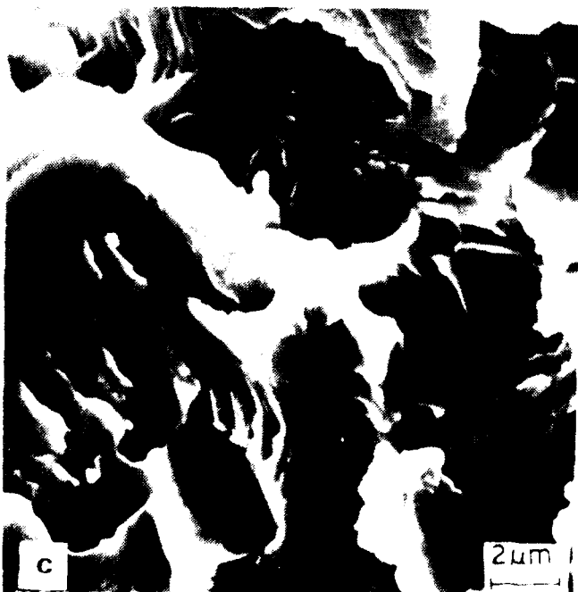
Figure 20 SEM fractographs of beta solutioned \text{Ti}_3\text{Al} fatigue crack growth specimen tested in vacuum at 1000°F.
