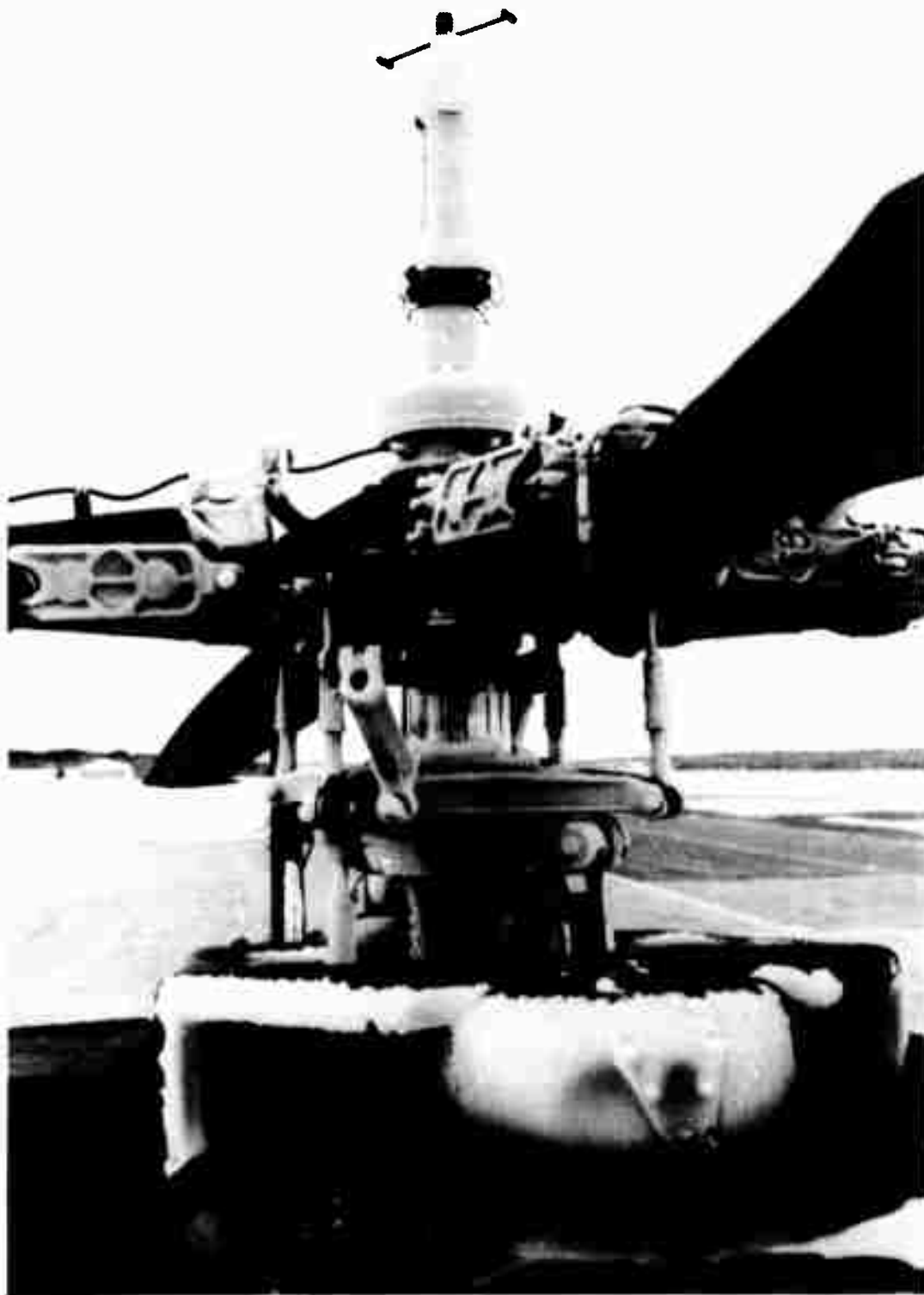
Photo 2. Residual Ice Accumulation on Unprotected Main Rotor Head Components
