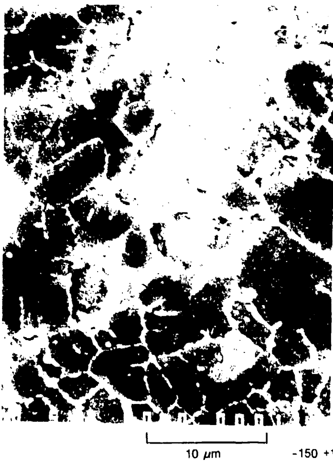
Figure 17. Microstructure of Fe_3Al + TiB_2 (724) Powder Particles — As-Produced
