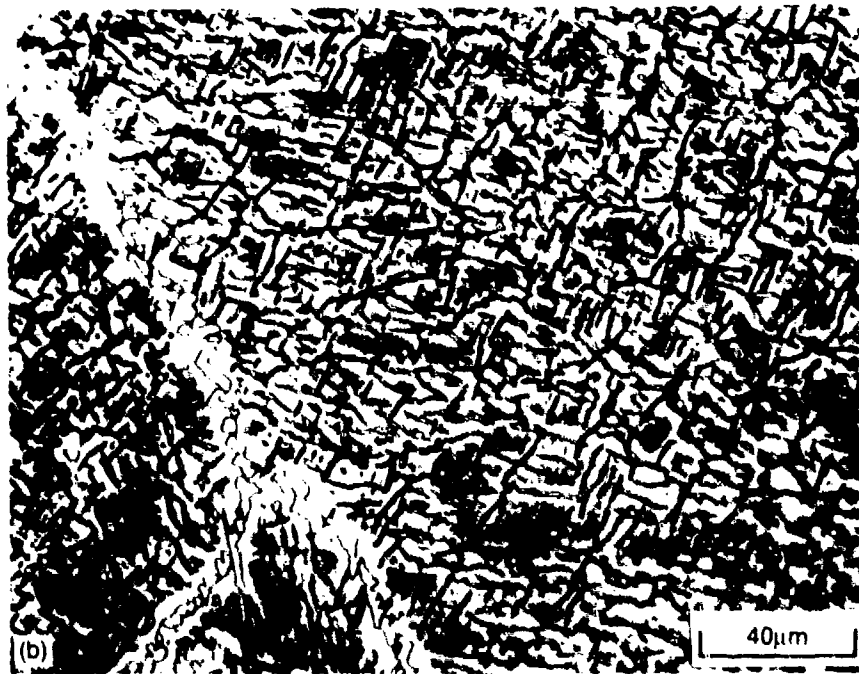
Figure 152. Microstructure of Alloy 155 After Heat Treatment at 1095°C for 1 Hour Followed by Cooling to 815°C at an Average Rate of About 2.5°C Per Minute. Note the Rapid Coarsening of the Modulated Structure During the Slow Cooling from 1095°C
