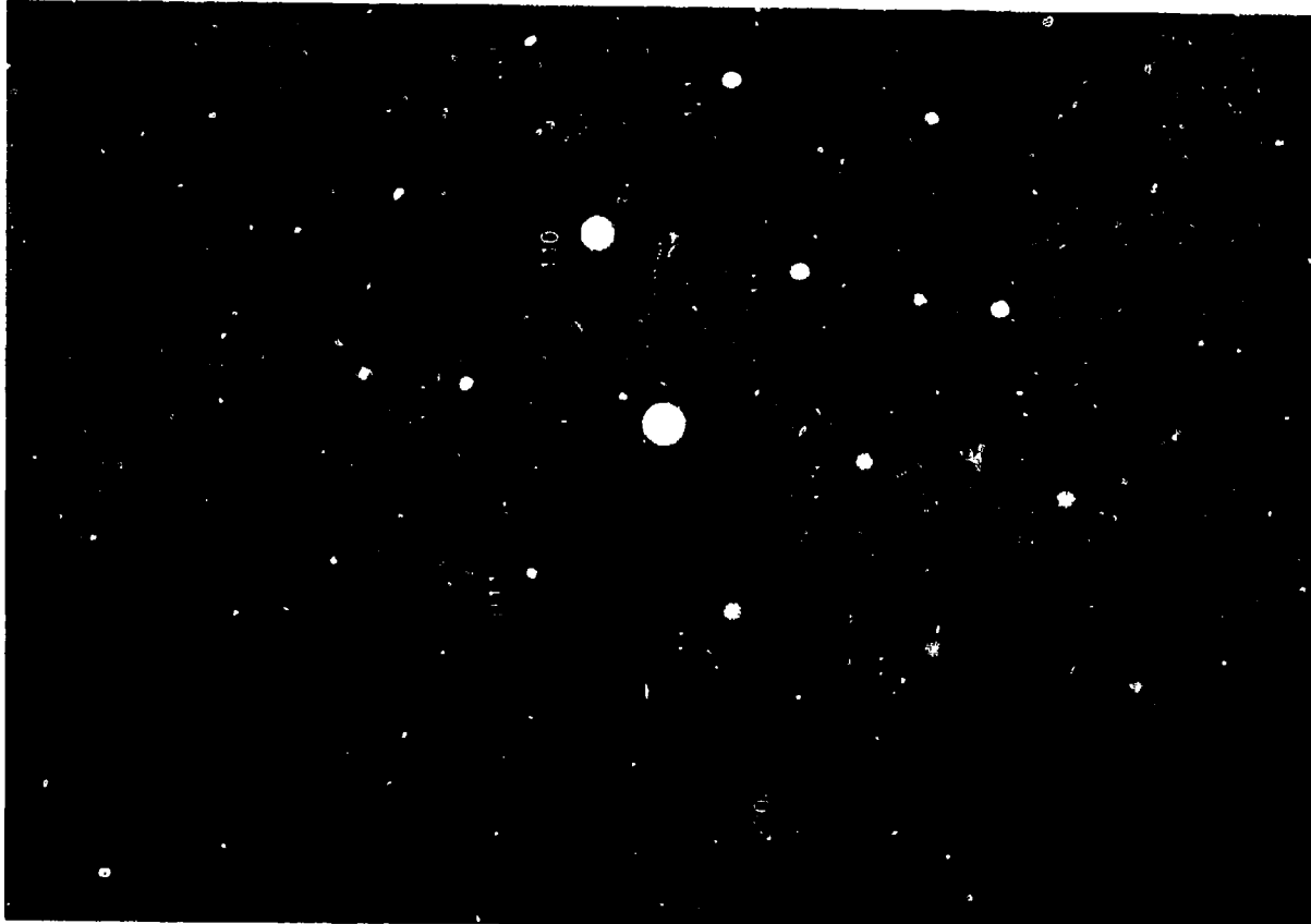
(111) Zone Axis FeAl B2 Structure: Recrystallized Areas With Abnormal Grain Growth
