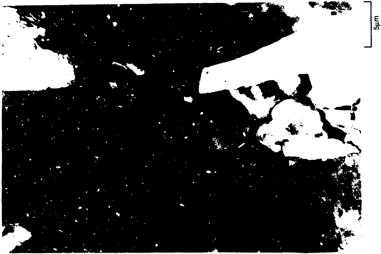
Figure 33. TEM of Fe 3 Al (729) Alloy Consolidated, Post Worked and Annealed at 1200°F (649°C) — Polygonized Area, Partially Recrystallized
