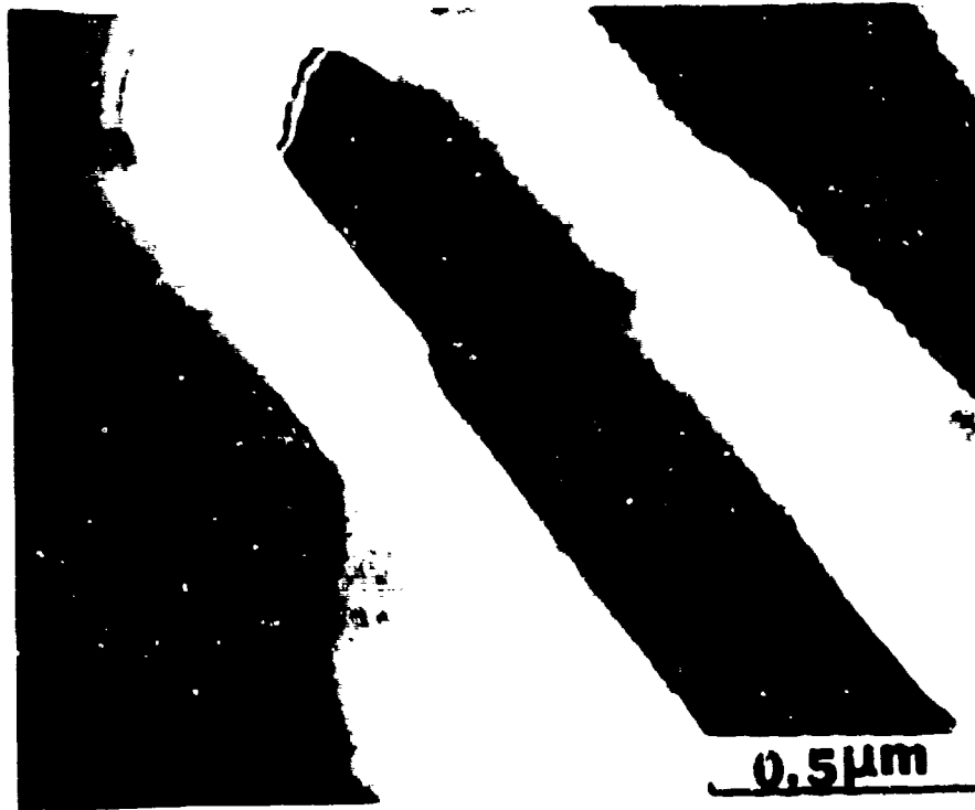
Figure 143. Electron Micrograph of the Lamellar Structure at Grain Boundary Regions in Alloy 97. The Dark and Light Phases Were Identified, Using Microelectron Diffraction Techniques, as Perovskite Carbide and Ferrite, Respectively
