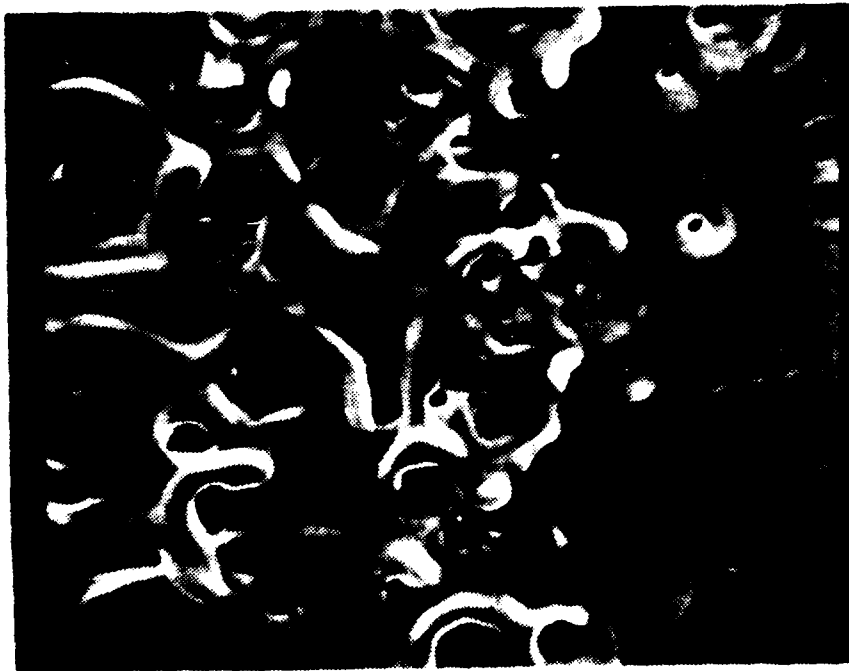
Figure 4.2 Boundary Region for Melting on Aluminum Target, 1200X, SEM
