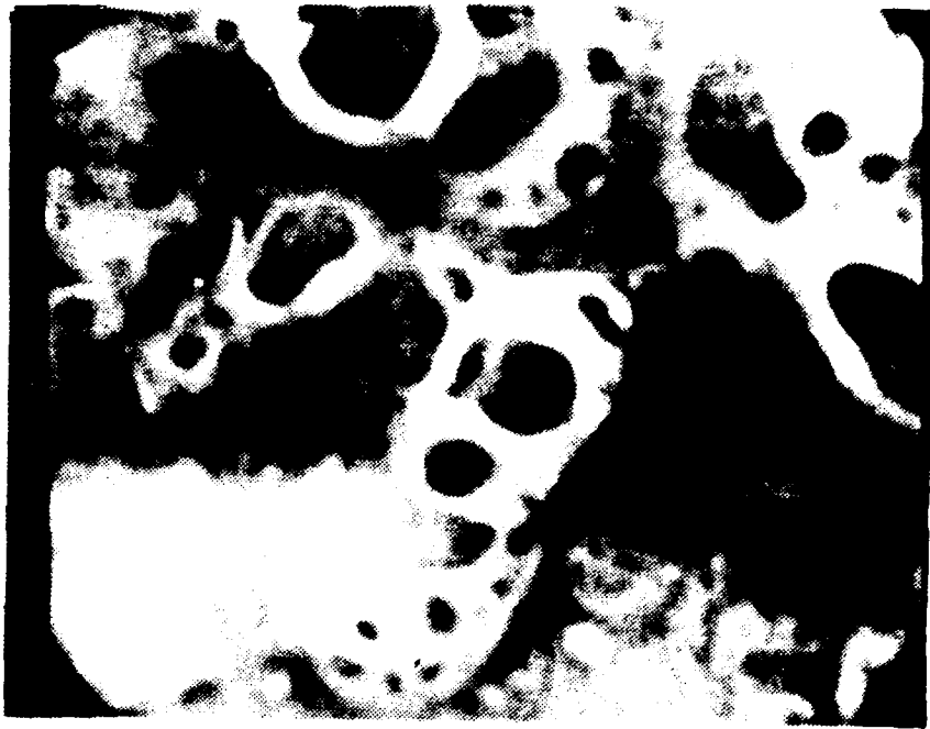
Figure 4.16 Barnacle-like Structures Appearing in Hot Spots, 7500X, SEM
