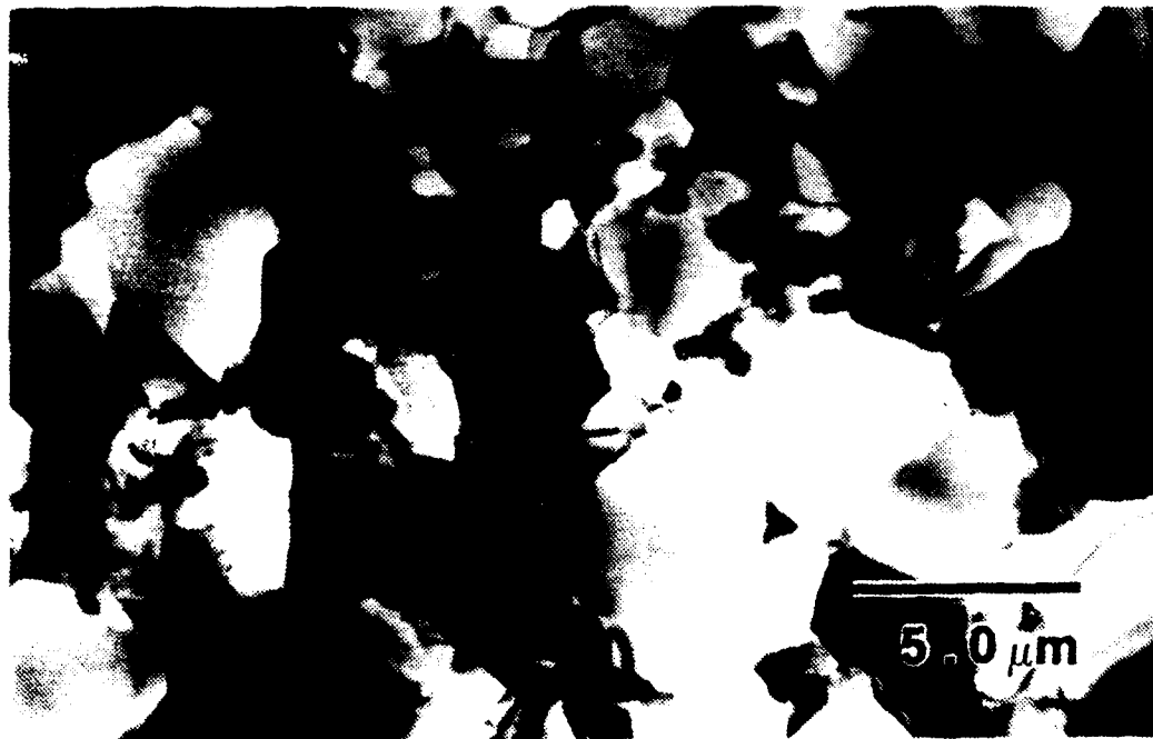
Figure 4.23 TEM Micrograph of an Al-10Mg-0.1Zr Alloy Processed by TMP2 and Annealed for 42 Hours
