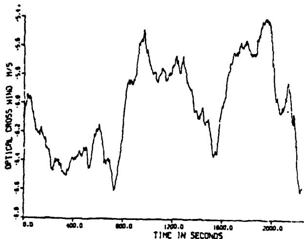
Fig. 5. The cross-path wind component from the 1 km optical path nearest the transmitter. The negative values mean that the wind is from the west. Data are from the entirety of Tape 24 of Session 1. The data is sampled every 2.56 s.
