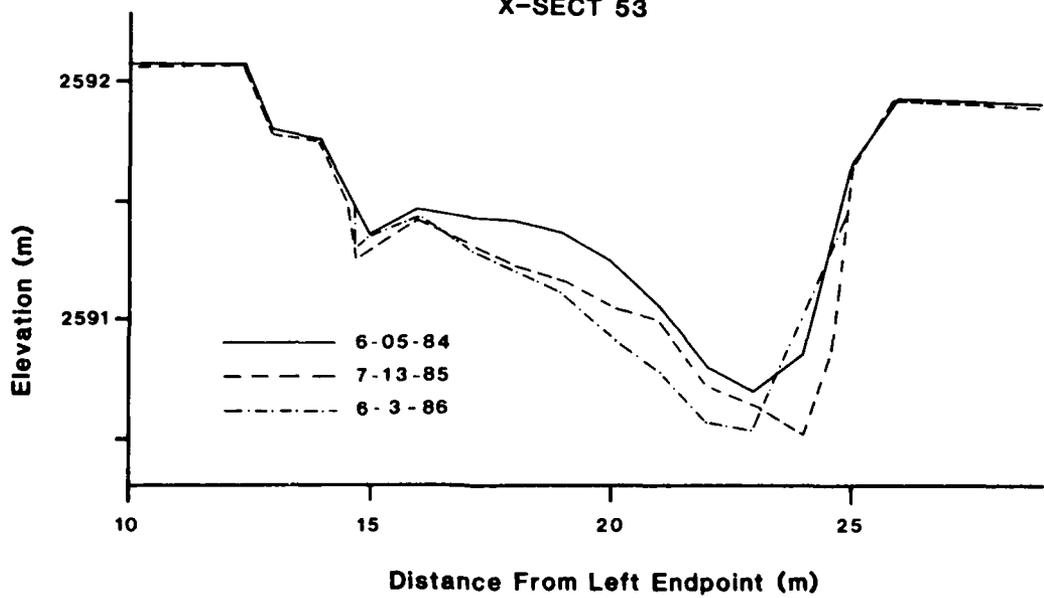
Figure 8. Channel cross sections downstream of the U.S. Highway 34 bridge.
