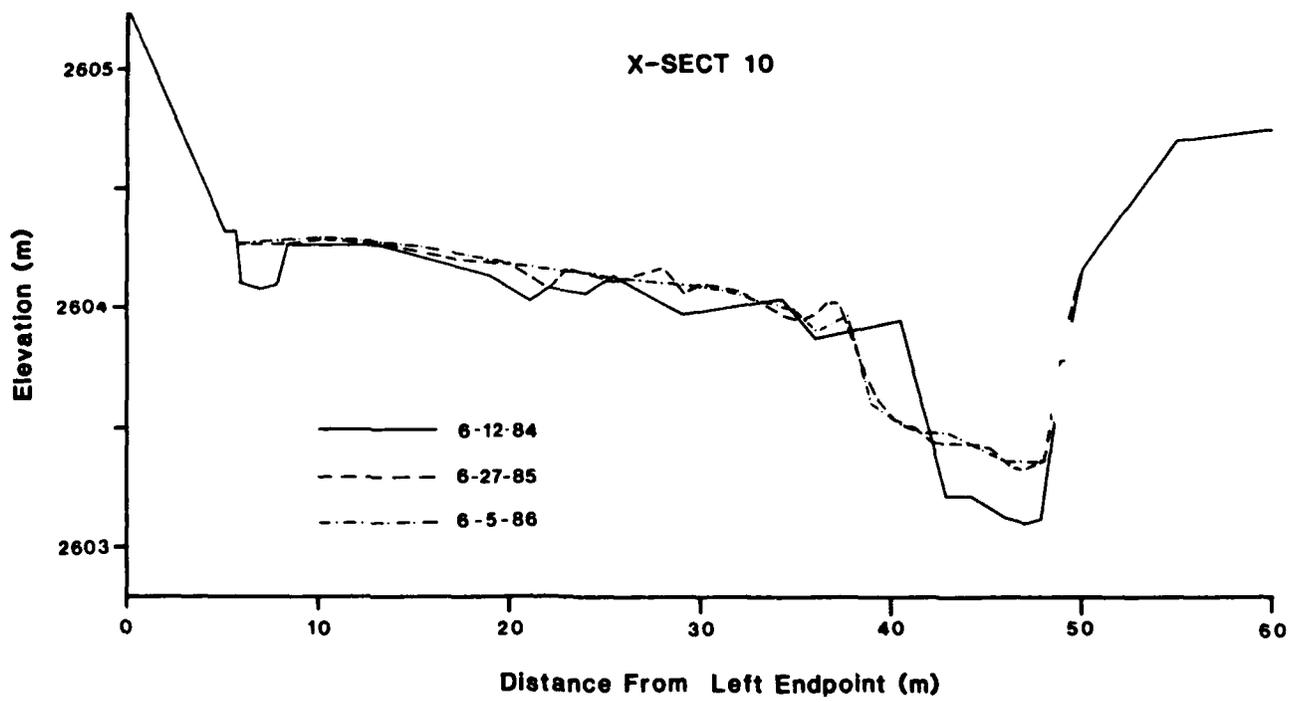
**Figure 6. Channel cross sections on the alluvial fan.**
