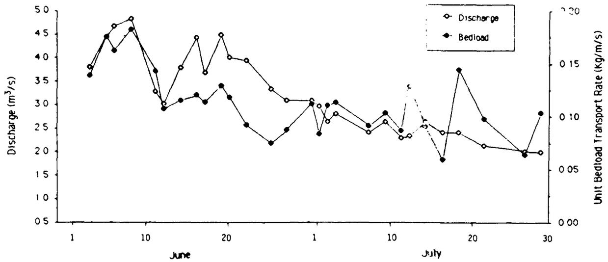
Figure 10. Comparison of water and bed load discharge at Cross Section 57 during the 1986 snowmelt period.
