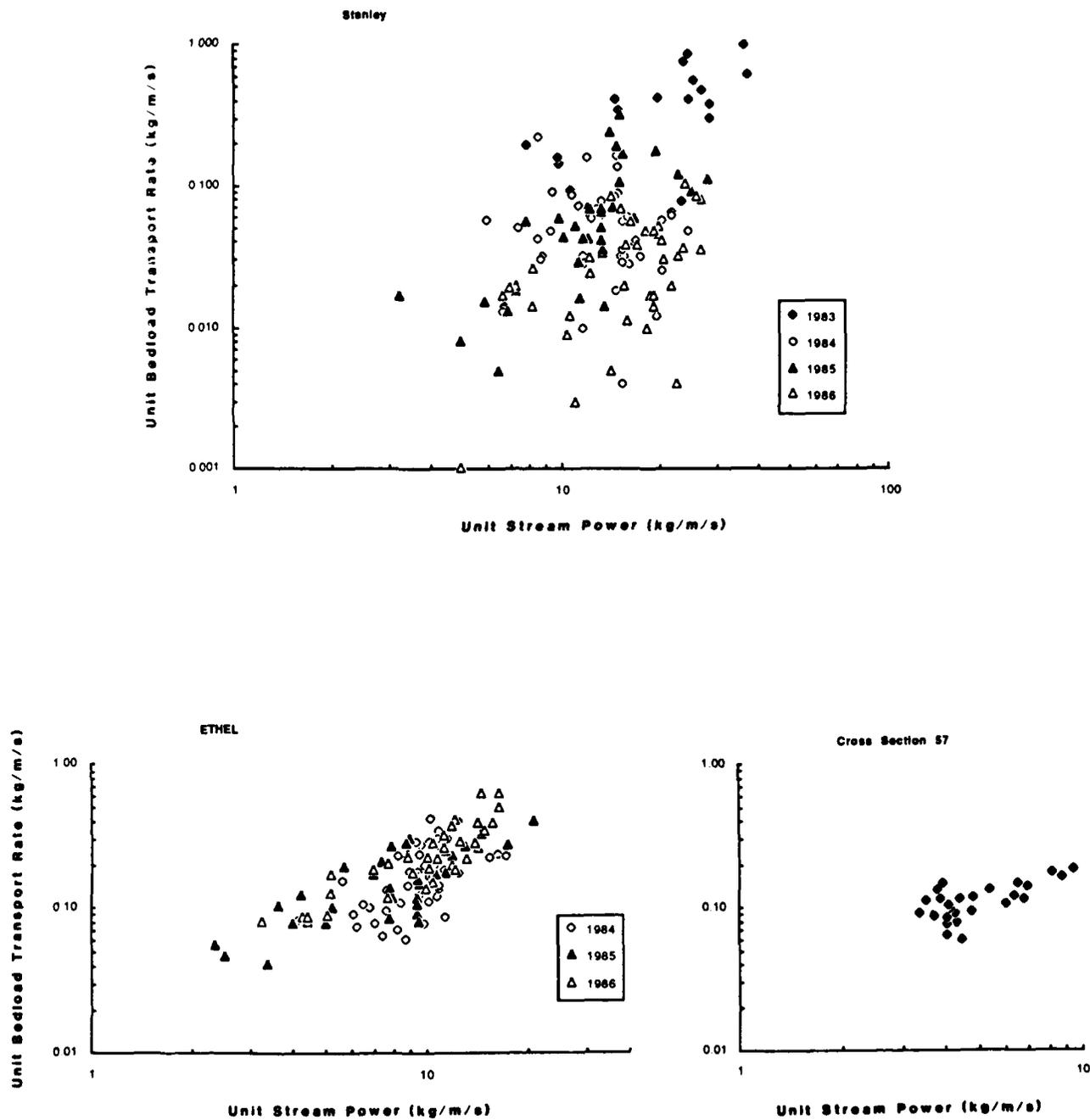
Figure 5. Sediment rating curves for the 3 Fall River sediment sampling sites.
