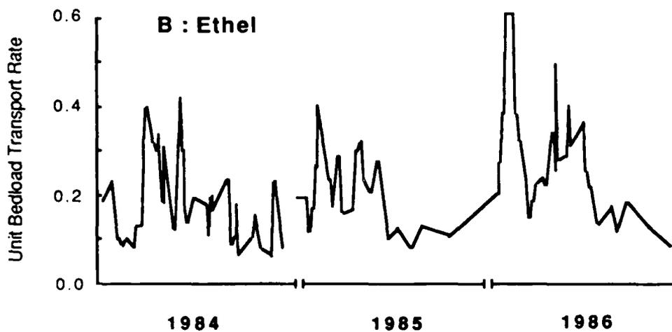
Figure 16. Trends in bedload transport rates as measured at two Fall River sampling sites. Data for Stanley includes measurements for the snowmelt runoff periods from 1983 through 1986; Data for Ethel includes measurements for the snowmelt runoff periods from 1984 through 1986.
