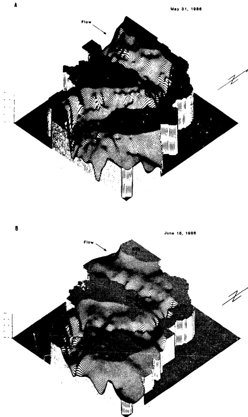
Figure 12. Isometric projection of bed topography within two bends of the storage zone reach (A) prior to the peak of snowmelt, May 31, 1986 and, (B) during the peak of snowmelt, June 18, 1986. Several cross section locations are shown for reference to Figs. 16 and 20. Note the growth of point bars between surveys.
