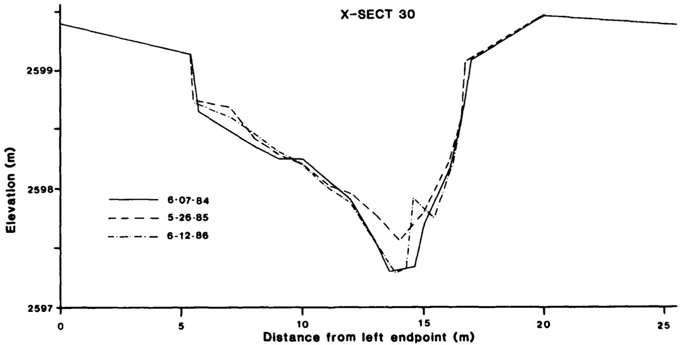
**Figure 7. Channel cross sections within the reach immediately downstream of the alluvial fan.**
