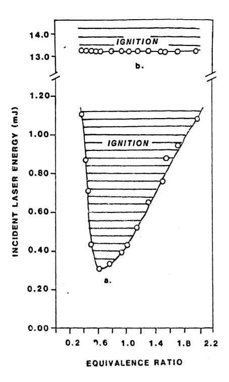
Figure 3. Dependence of the Incident Laser Energy Required to Ignite a H<sub>2</sub>/O<sub>2</sub> Nixture as a Function of Equivalence Ratio (a) For the Laser Wavelength Set at the Peak of the O-Atom Two-Photon Excitation, (b) For the Nd:YAG Second Harmonic (532 nm)
