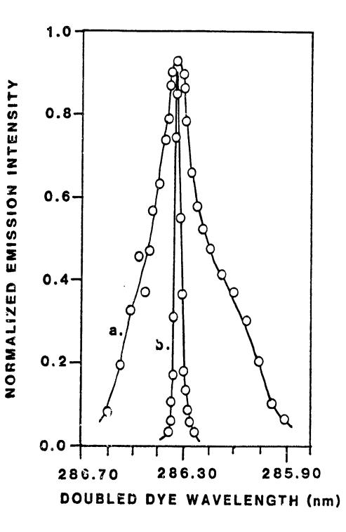
Figure 4. Excitation Curve for O-Atom Emission at 777.5 nm from (a) an  $O_2$  Flow, (b) : Stoichiometric  $H_2/O_2$  Flame
