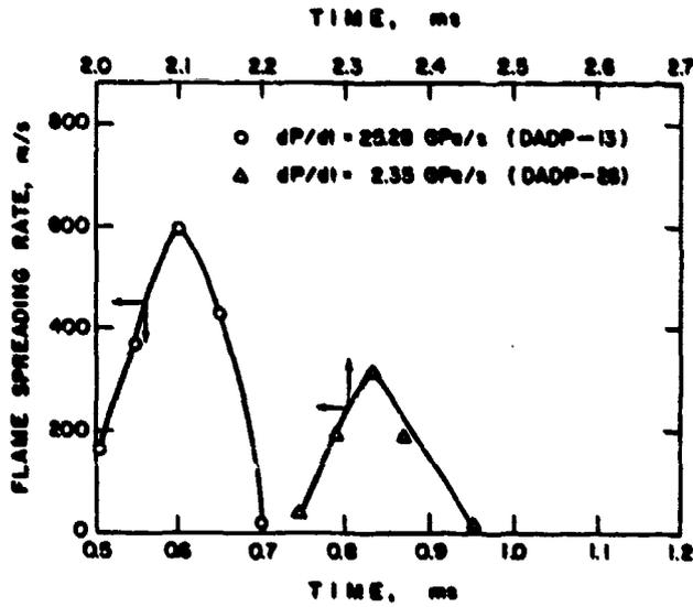
Fig. 13 Flame Spreading Rates under Different Pressurization Rates
