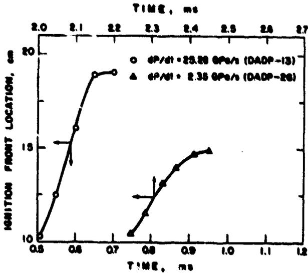
Fig. 12 Flame-Front Trajectories for Different Pressurization Rates
