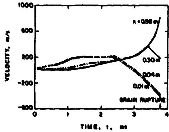
Fig. 15 Calculated Velocity-Time Traces at Various Axial Locations
