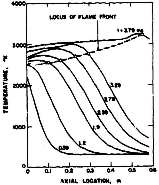
Fig. 19 Calculated Temperature Distribution at Various Times
