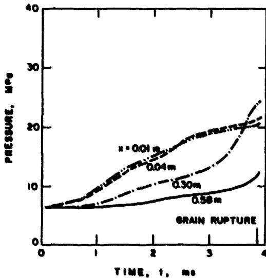
Fig. 14 Calculated Pressure-Time Traces at Various Axial Locations
