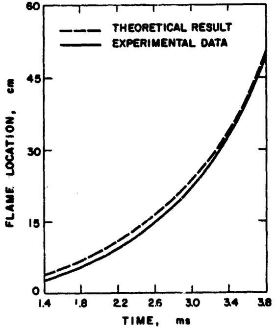
Fig. 23 Comparison of Calculated and Measured Flame-Front Locations
