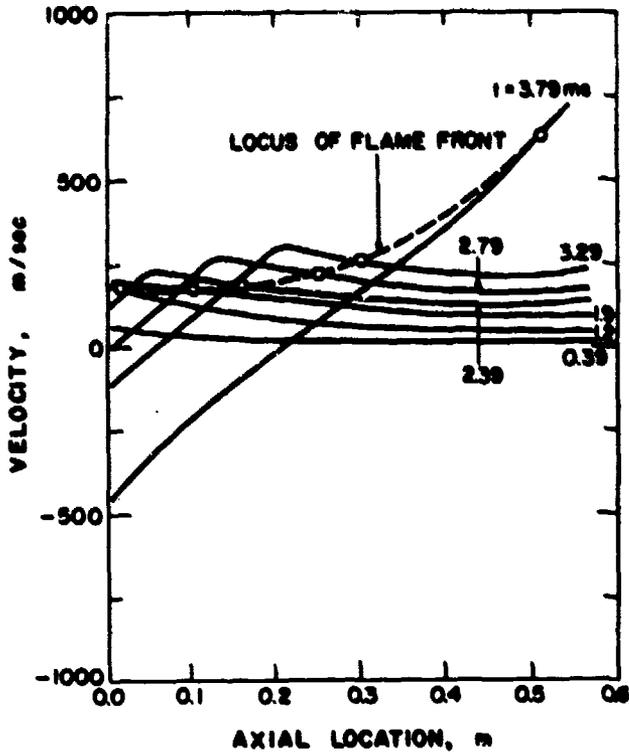
Fig. 18 Calculated Velocity Distribution at Various Times
