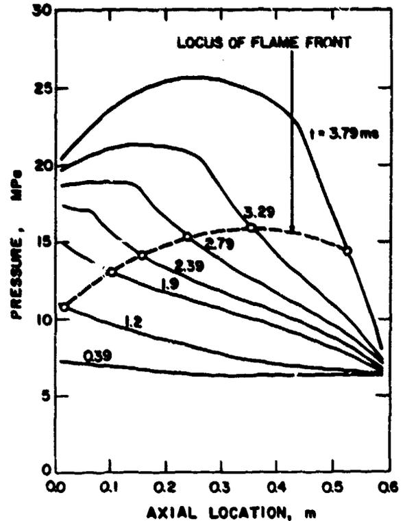
Fig. 17 Calculated Pressure Distribution at Various Times
