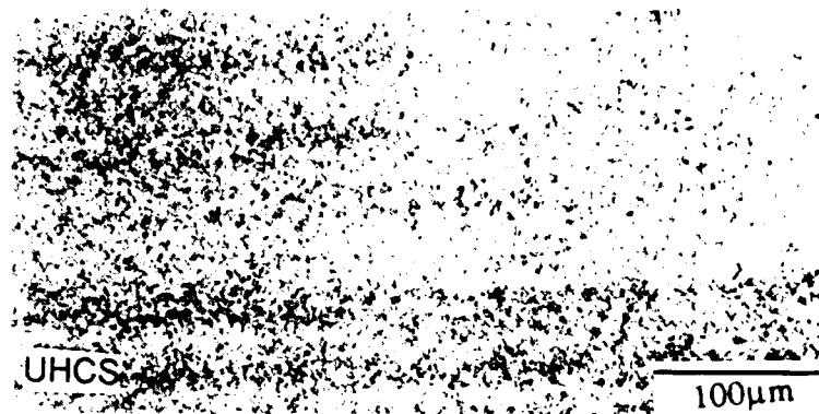
Figure 8. Interface structure of the 26Cr-1Mo / Cu / UHCS-1.6Al laminated elongated 300% at 775° C. Despite time and strain at elevated temperature, no cavitation or interdiffusion are visible at the interface of this laminated composite.
