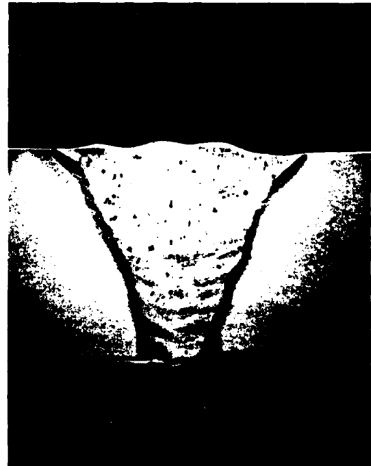
Fig. 1—Cross section of underwater wet weld.
