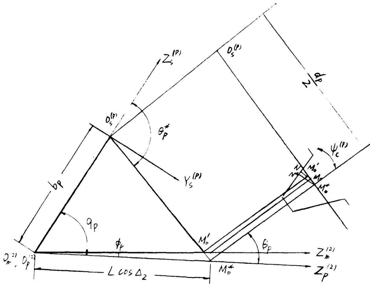
$M_0'$  is the intersection of the pitch line and  $\overline{O_s^{(1)} M_0^*}$
