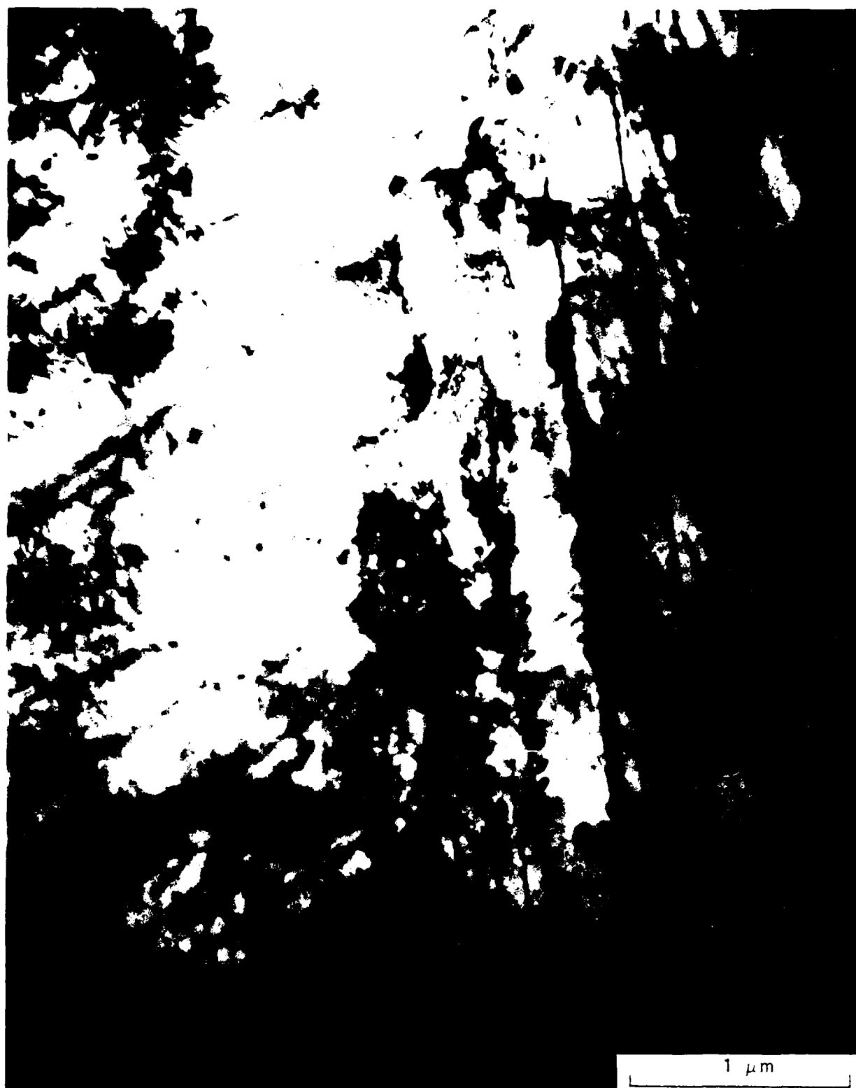
Fig. 15 Transmission Electron Micrograph of Prior \beta -Grain Boundary Region in Ti-6211 Specimen EYL-1797. Note chain of precipitates near edge of grain boundary
