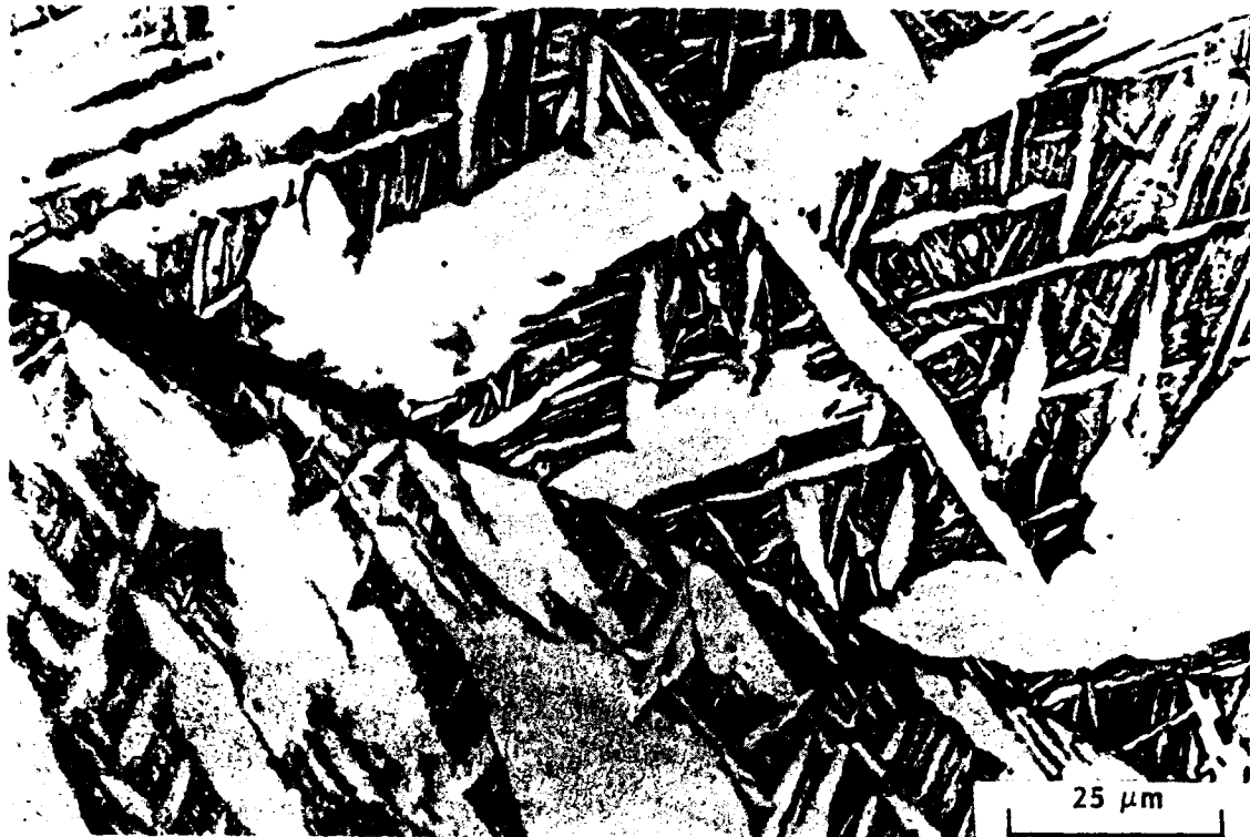
Fig. 45 Optical Micrograph of Ti-6211 Hot Ductility Specimen FQC-52 Showing Numerous Small Microvoids Within the Prior Beta Grains as Well as Crack Growth Along a Prior Beta Grain Boundary
