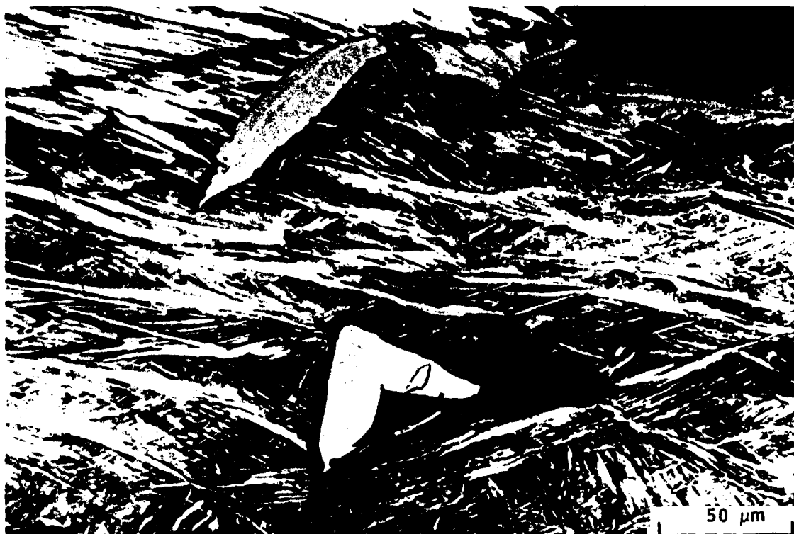
Fig. 46 Optical Micrograph of Ti-6211 Hot Ductility Specimen FQC 52 Showing a Large Microvoid Formed in the Matrix Adjacent to Large Lenticular Martensite. Note the irregular-shaped twin within the latter
