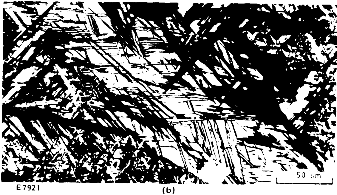
Fig. 50 Optical Micrograph of Ti-6211 Specimen FQC-5b After Hot Ductility Testing About 60 C (108 F) Below the Beta \rightarrow Alpha Transformation Temperature Range, (a) Bright Field, (b) Polarized Light. Note the extensive twinning present, revealed clearly in (b)
