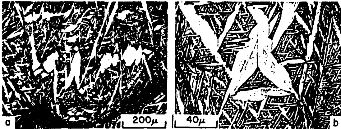
Fig. 1 - Light micrographs showing, (a) three types of transformation products and (b) higher magnification of a pair of large plates.
