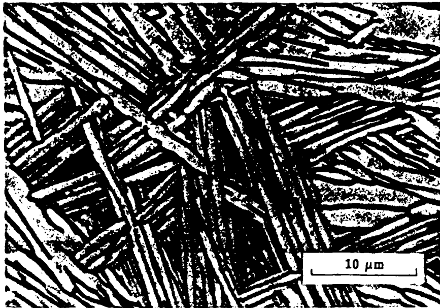
Fig. 7: Optical micrograph of Widmanstatten alpha plus beta microstructure in the fusion zone of the weldment produced from weld wire containing high boron. Etchant is HF-alcohol.
