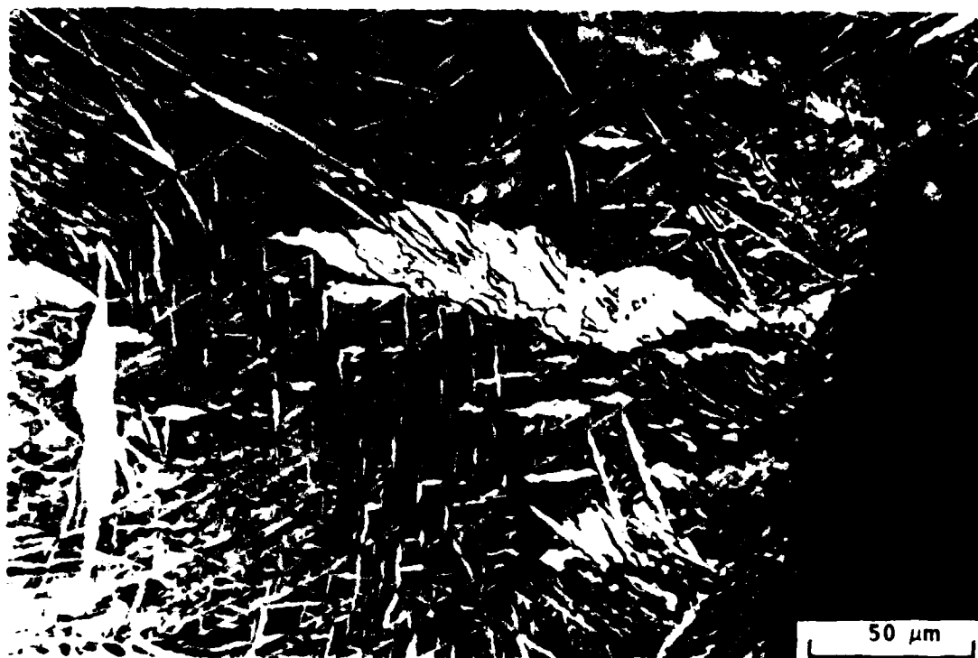
Fig. 52 Optical Micrograph of Ti-6211 Specimen FQC-46 After Hot Ductility Testing. Note the irregular shape of deformation twins in the large, clear-etching patch (massive alpha)
