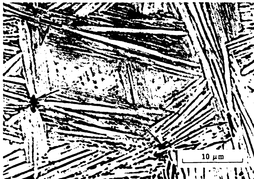
Fig. 9: Optical micrograph of microstructure in fused end of welding wire containing high boron. The dark appearing particles (see arrows) have been tentatively identified as TiB.
