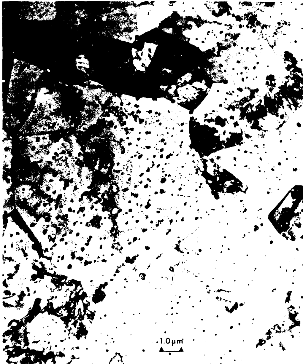
GRAIN STRUCTURE AND GADOLINIA DISTRIBUTION Ti-11Al-0.5Gd (at%) 125 \mu m THICK SPLAT; AGED AT 800°C/0.25 hr
