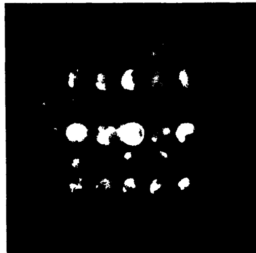
[100] CONVERGENT BEAM MICRODIFFRACTION PATTERN FROM DYSPROSIA PRECIPITATE, 40 nm SPOT SIZE
