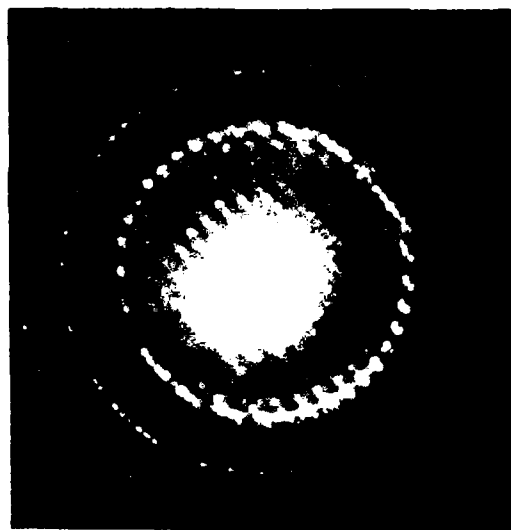
SADP; MONOCLINIC ZONE AXIS: [1\bar{3}2] POINTER MARKS g OF DARK FIELD IMAGE
