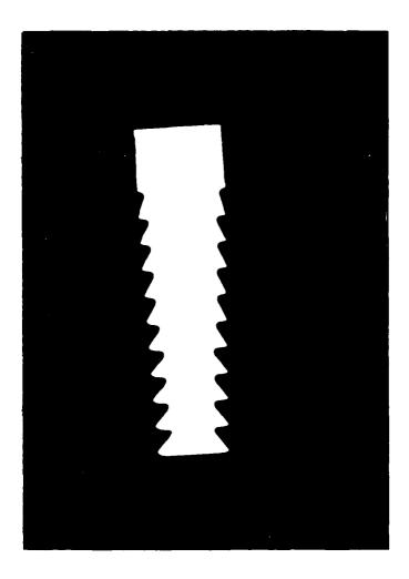
FIGURE 1. SERRATED ALUMINUM OXIDE DENTAL IMPLANT
