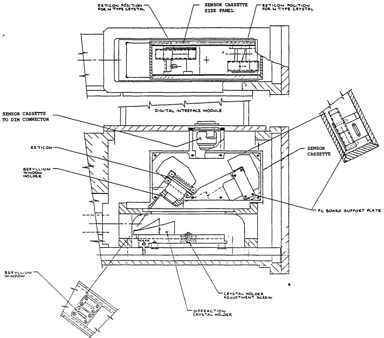
Figure 6. Layout design of the detector package.
