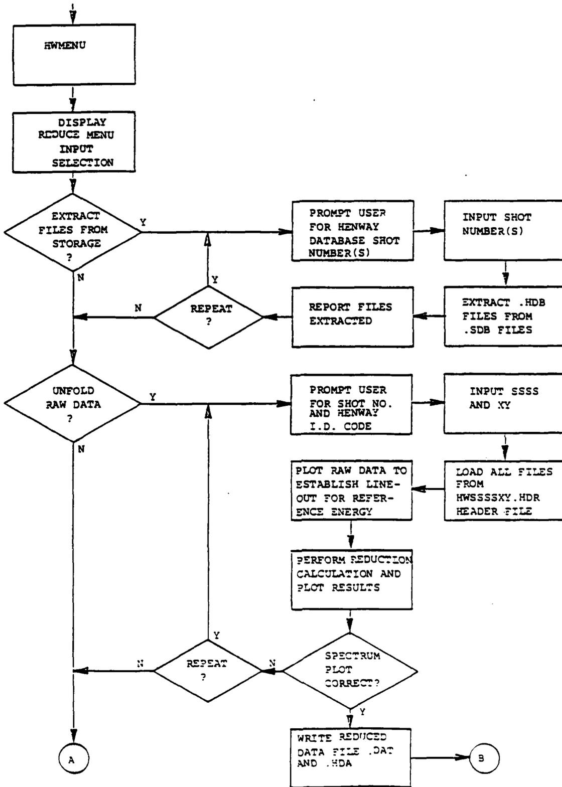
Figure 21. REDUCE control flow.
