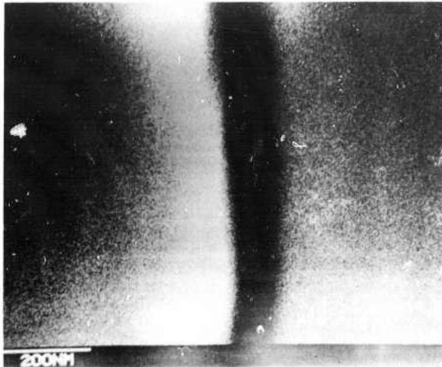
Figure 25 SEM photograph of the smallest source image made with UV lithography, demonstrating the feasibility of fabricating a quarter micron wide source electrode with UV radiation of 436 nm.
