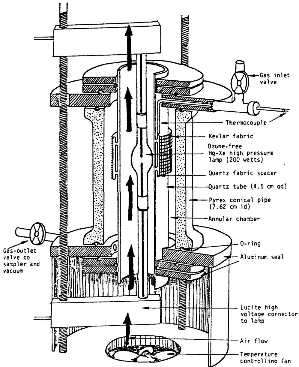
FIGURE 2. Schematic Longitudinal Section of Photolysis Chamber.
