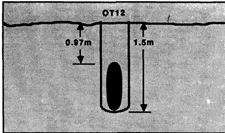
Figure 4. The installation of the 155-mm shell in hole OT12.
