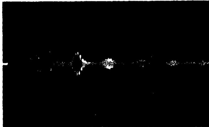
Fig. 28 — Experimental observation of a "slow" circumferential wave at  $k_0 a = 43$ , on a stainless steel shell. The time scale is  $20 \mu\text{s}/\text{division}$ ; the amplitude scale is  $2 \text{ mv}/\text{division}$ .
