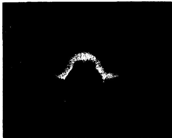
Fig. 29 — Schlieren visualization of a "fast" circumferential wave at  $k_0 a = 202$  on a stainless steel shell.
