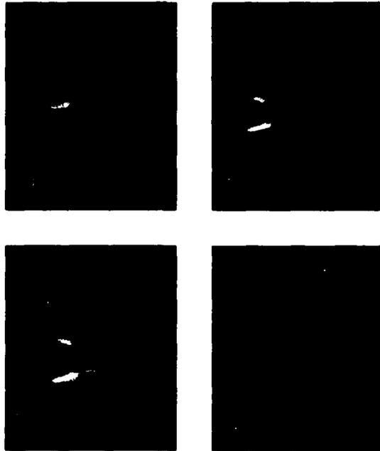
Fig. 12 — A time sequence of schlieren photographs showing the effect of illuminating a 0.002-cm-thick plate with an incoming acoustic pulse at  $\theta_i = 13.0^\circ$ . Pulse length is 3  $\mu$ sec; frequency is 7.2 MHz.
