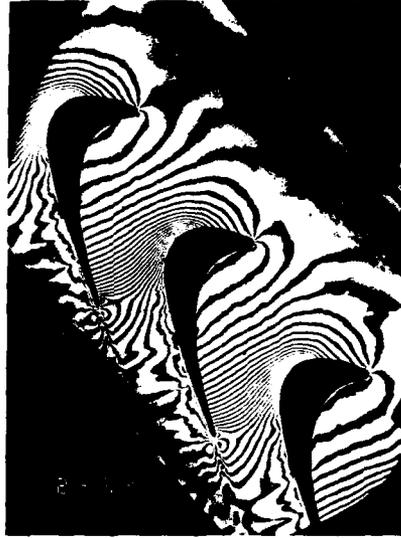
Fig 9. Absolute hologram of cascade
