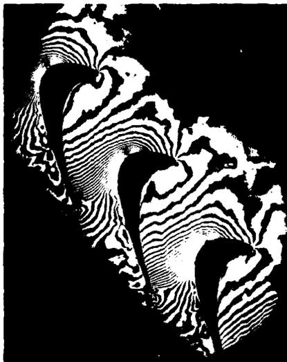
Fig 6. Absolute hologram of cascade
