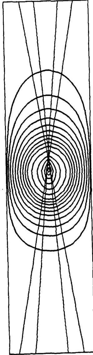
Fig. 6 Temperature contours for laser power of 720 W and inlet velocity of 0.01 m/s.  $T_{MAX} = 16,863$  K;  $\Delta T = 1000$  K.
