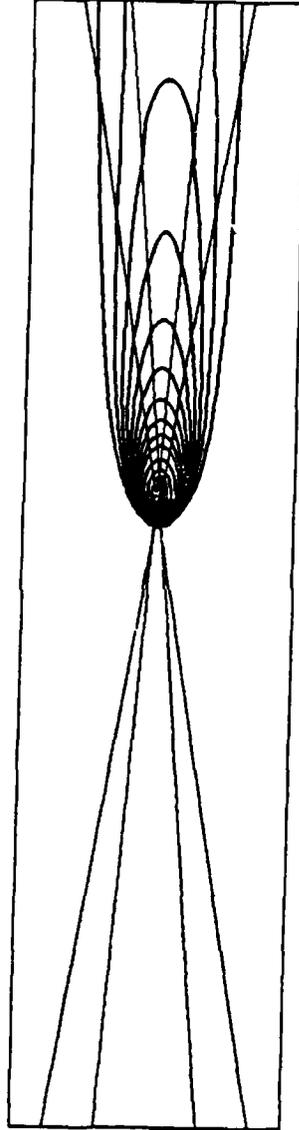
Fig. 4 Temperature contours for laser power of 720 W and an inlet velocity of 1.0 m/s.  $T_{MAX} = 17,809$  K;  $\Delta T = 1000$  K.
