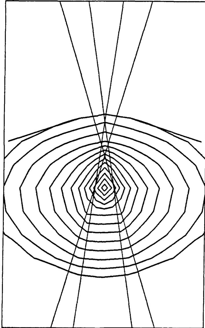
Fig. 7 Close-up view of temperature contours near focal point for case shown in Fig. 6.  $\Delta T = 500$  K.
