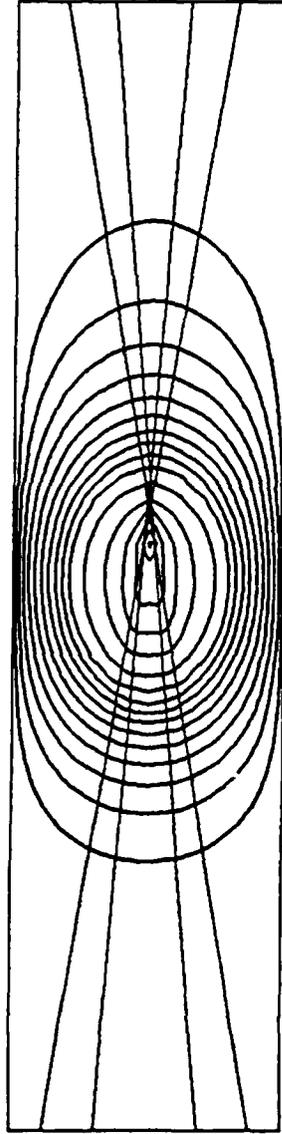
Fig. 9 Temperature contours for laser power of 1000 W and inlet velocity of 0.01 m/s.  $T_{MAX} = 16,246$  K;  $\Delta T = 1000$  K.
