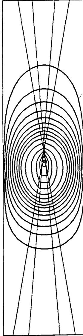
Fig. 8 Temperature contours for laser power of 900 W and inlet velocity of 0.01 m/s.  $T_{MAX} = 16,593$  K;  $\Delta T = 1000$  K.
