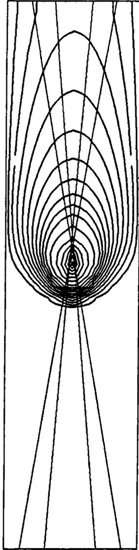
Fig. 5 Temperature contours for laser power of 720 W and inlet velocity of 0.15 m/s.  $T_{MAX} = 17,526$  K;  $\Delta T = 1000$  K.
