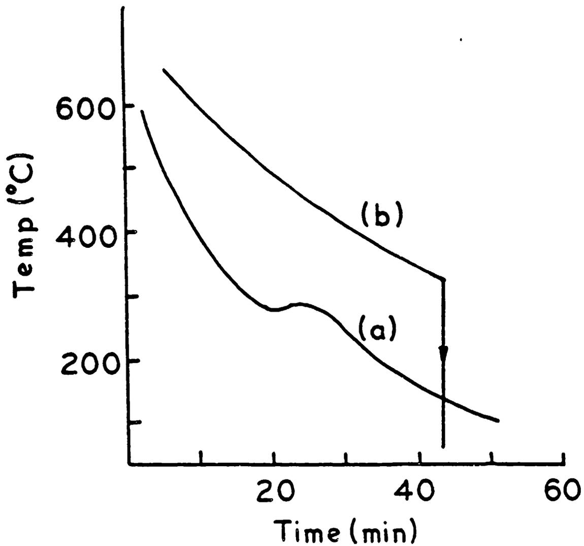
Figure 3. Slow-cooling experiments. Figure 3(a) shows the time-temperature path recorded for air cooling of a seven-pound disk after austenitizing. Figure 3(b) shows the path for an insulated disk which was water-quenched from just above the  $M_s$  temperature to avoid recalescence effects.
