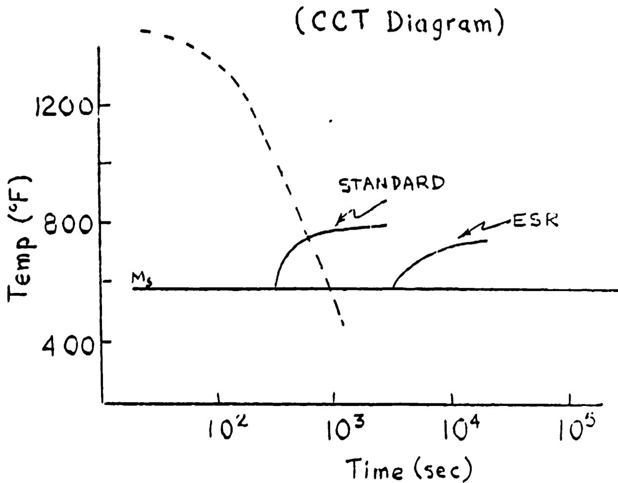
Figure 2. Continuous-cooling-transformation curves for ASTM A723 steels from different sources. The dashed line represents the cooling path used to obtain the data in Figure 1.
