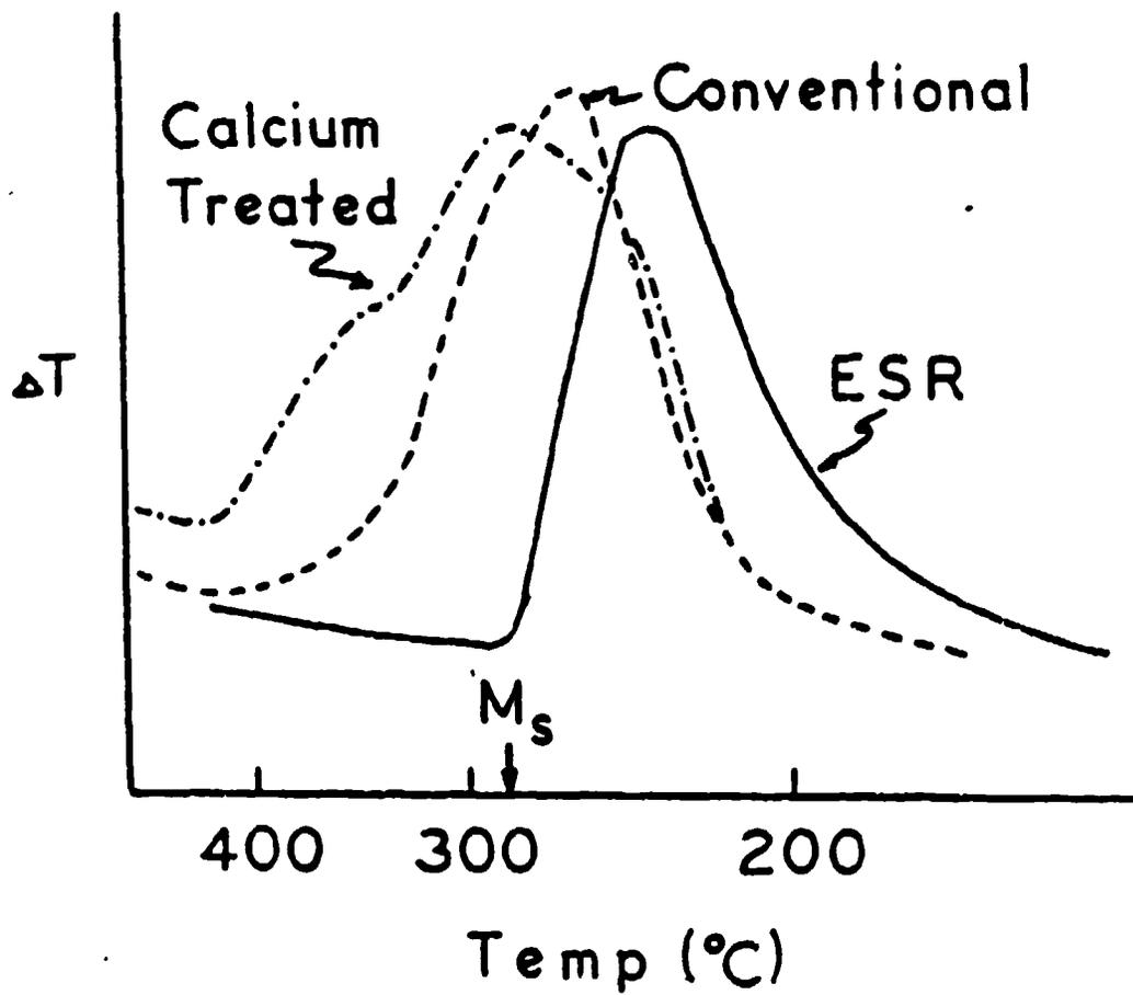
Figure 1. Differential thermal analysis output during continuous cooling of various ASTM A723 steels from the austenite temperature.
