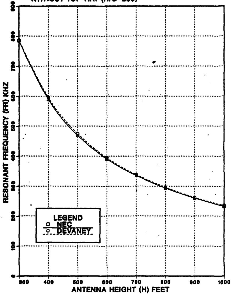
Figure 3.2 Variation of Resonant Frequency of Reference Antenna as a Function of Antenna Height.
