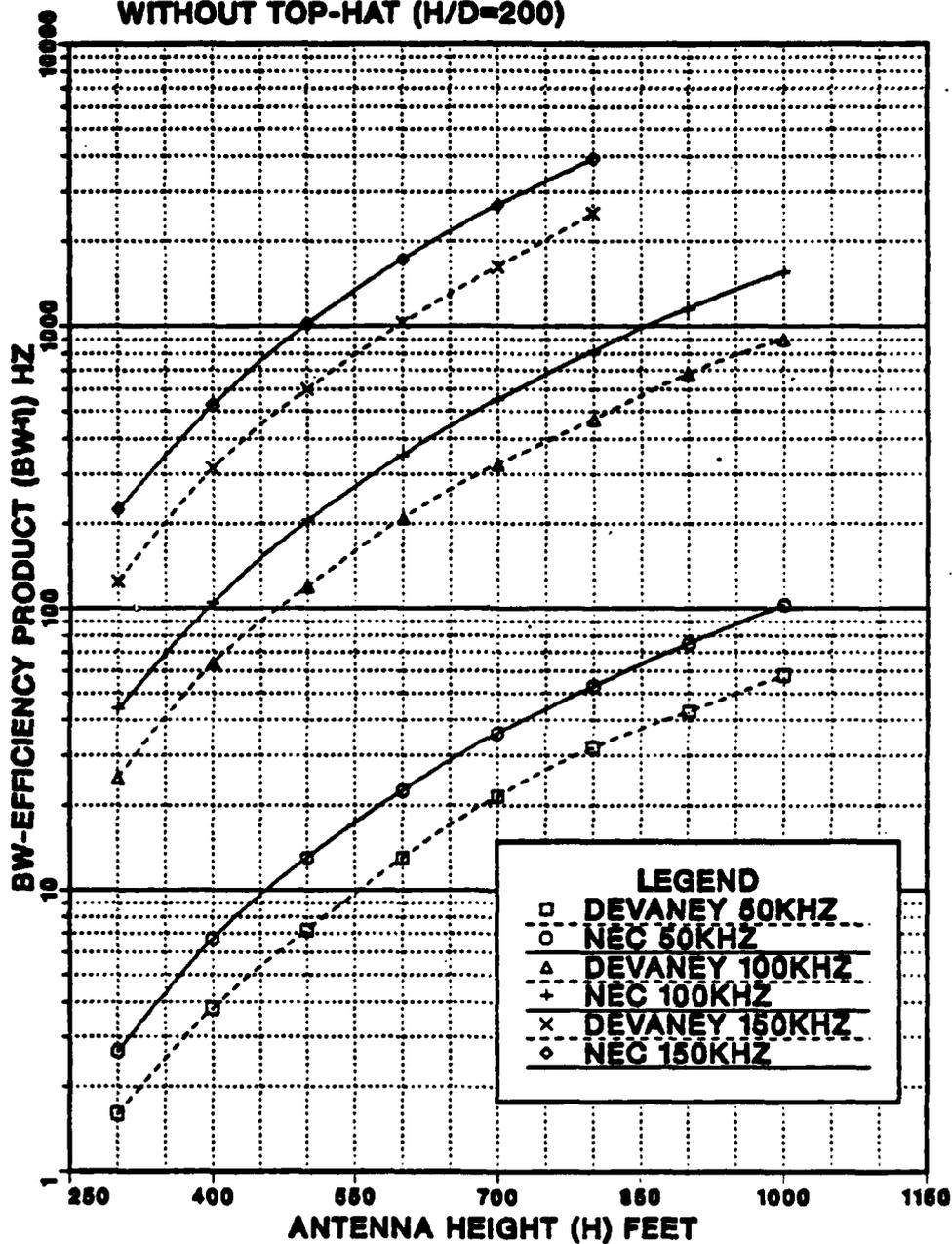
Figure 3.5 Variation of Reference Antenna Bandwidth-Efficiency Product as a Function of Antenna Height.
