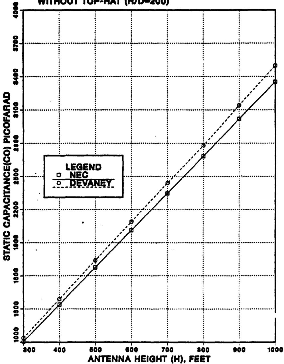
Figure 3.1 Variation of Static Capacitance of Reference Antenna as a Function of Antenna Height.
