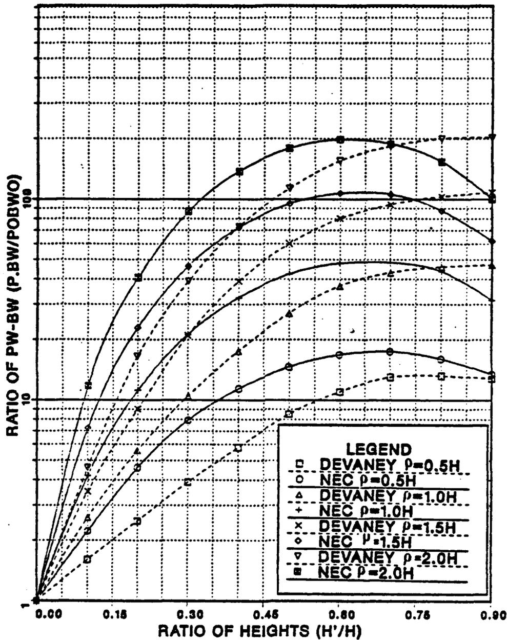
Figure 3.14 Normalized Power-Bandwidth Product of Top-Loaded Antenna, the Number of Top-Hat Radials  $N = 6$ .
