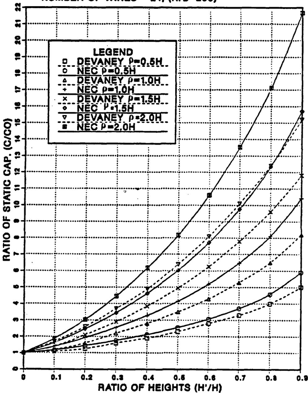
Figure A.8 Normalized Static Capacitance of Top-Loaded Antenna, the Number of Top-Hat Radials  $N = 24$ .
