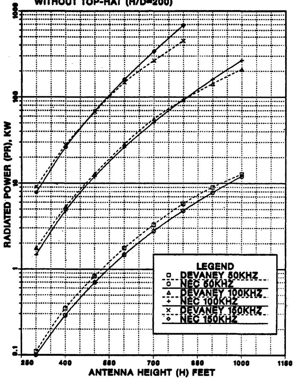
Figure 3.6 Variation of Reference Antenna Maximum Radiated-Power Capability as a Function of Antenna Height.
