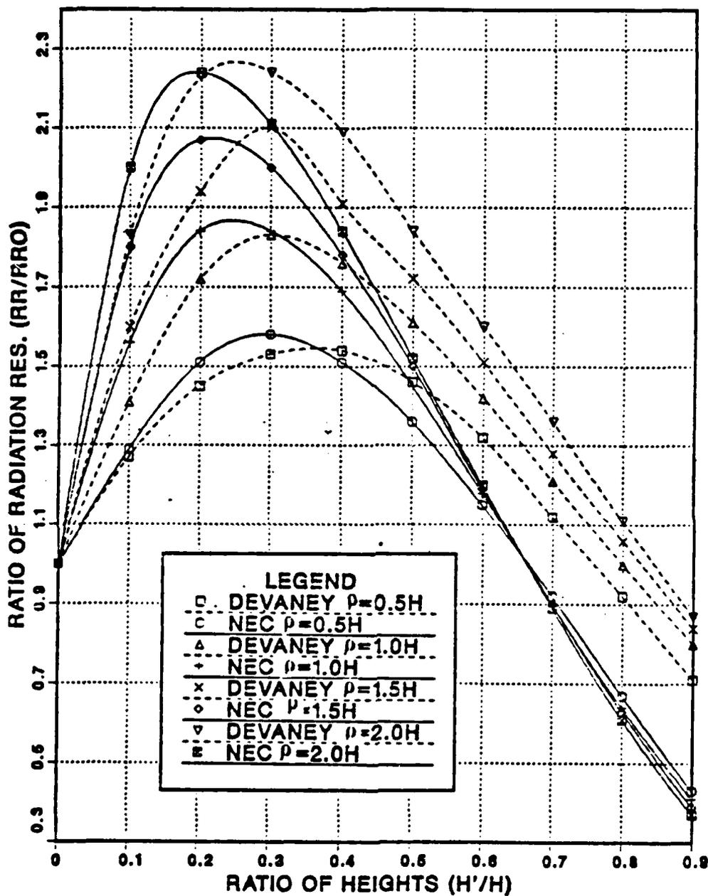
Figure A.4 Normalized Radiation Resistance of Top-Loaded Antenna, the Number of Top-Hat Radials  $N = 12$ .
