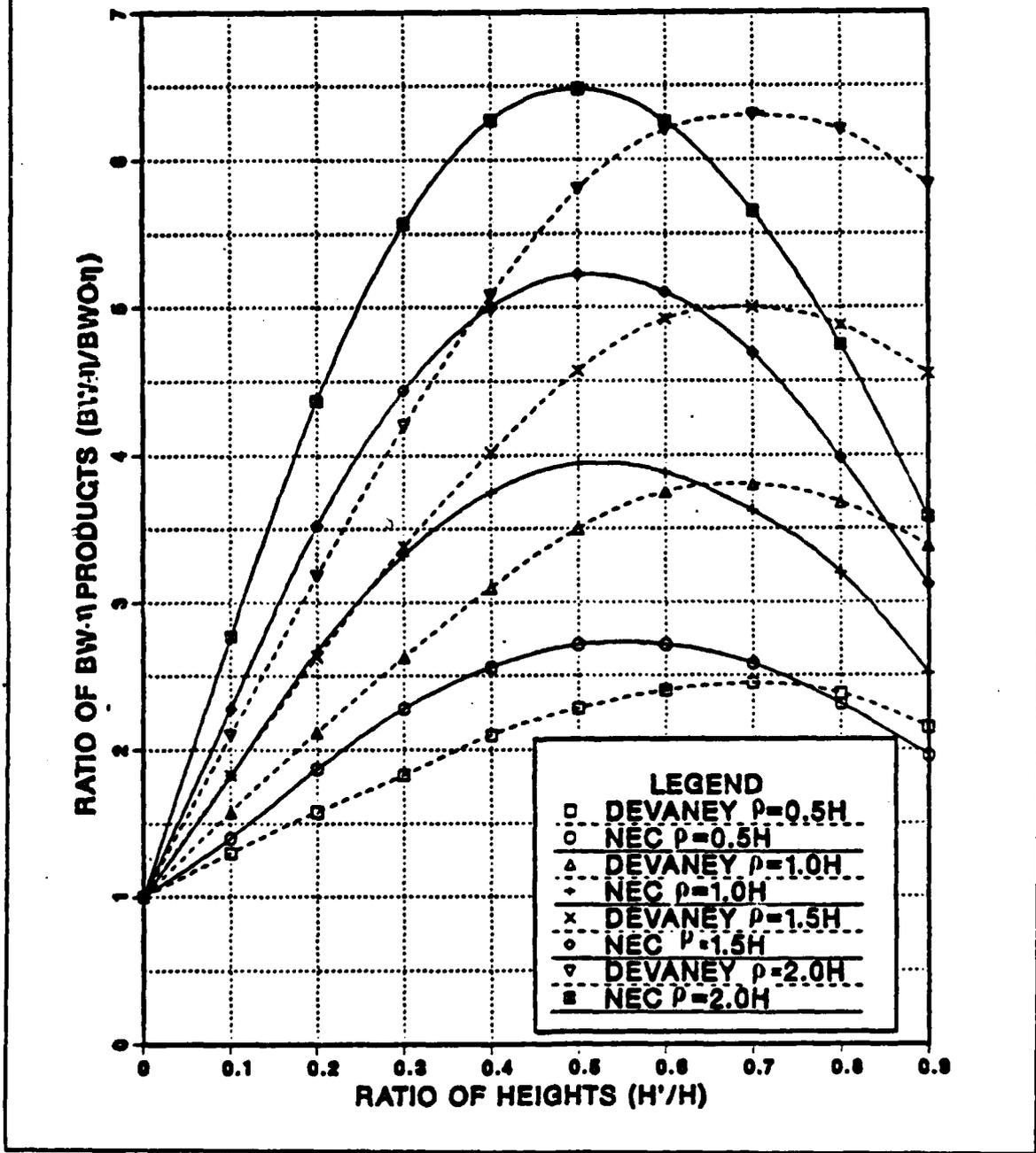
Figure 3.12 Normalized Bandwidth-Efficiency Product of Top-Loaded Antenna, the Number of Top-Hat Radials  $N = 6$ .
