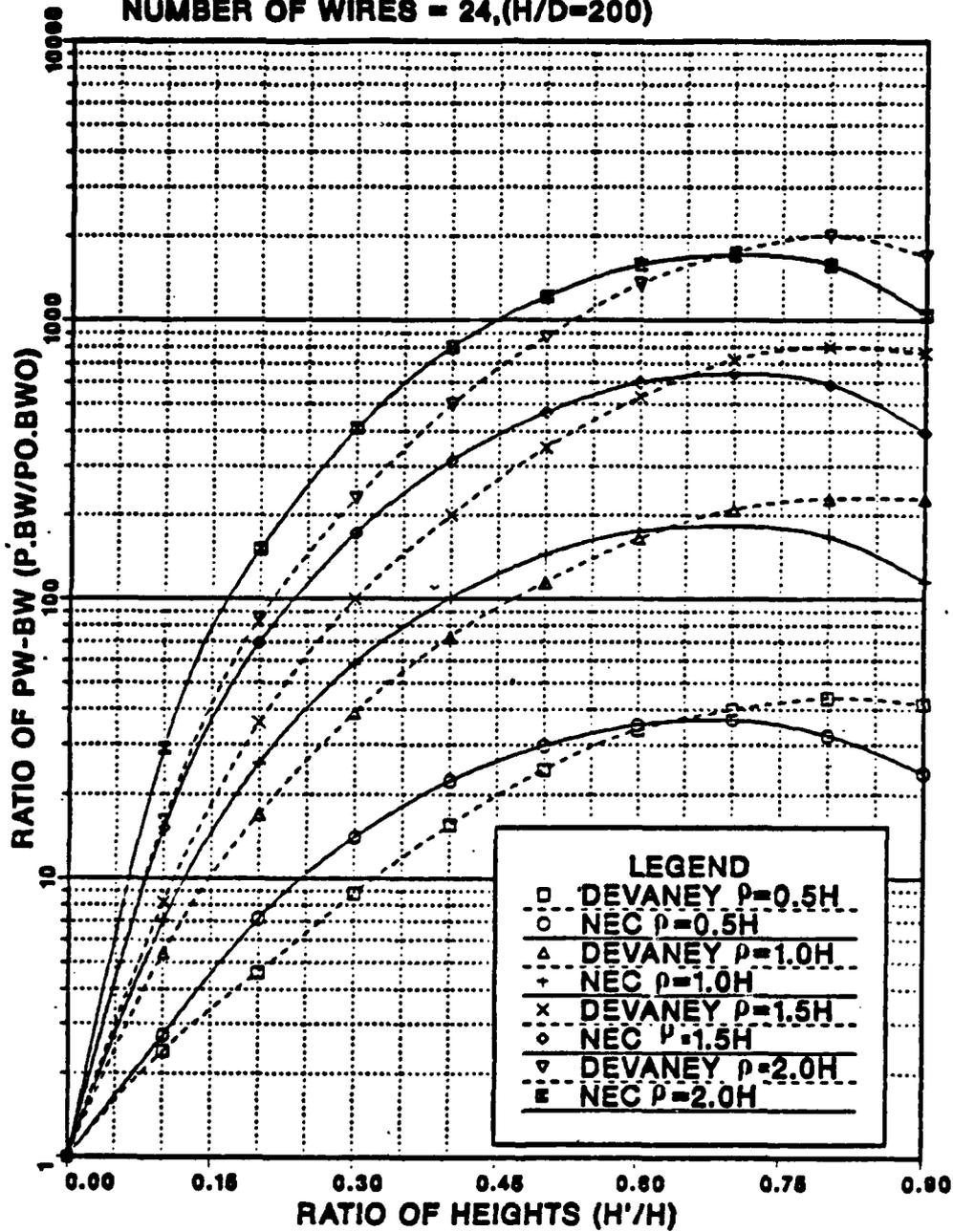
Figure A.14 Normalized Power-Bandwidth Product of Top-Loaded Antenna, the Number of Top-Hat Radials  $N = 24$ .
