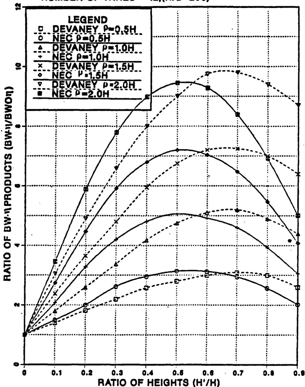
Figure A.5 Normalized Bandwidth-Efficiency Product of Top-Loaded Antenna, the Number of Top-Hat Radials  $N = 12$ .
