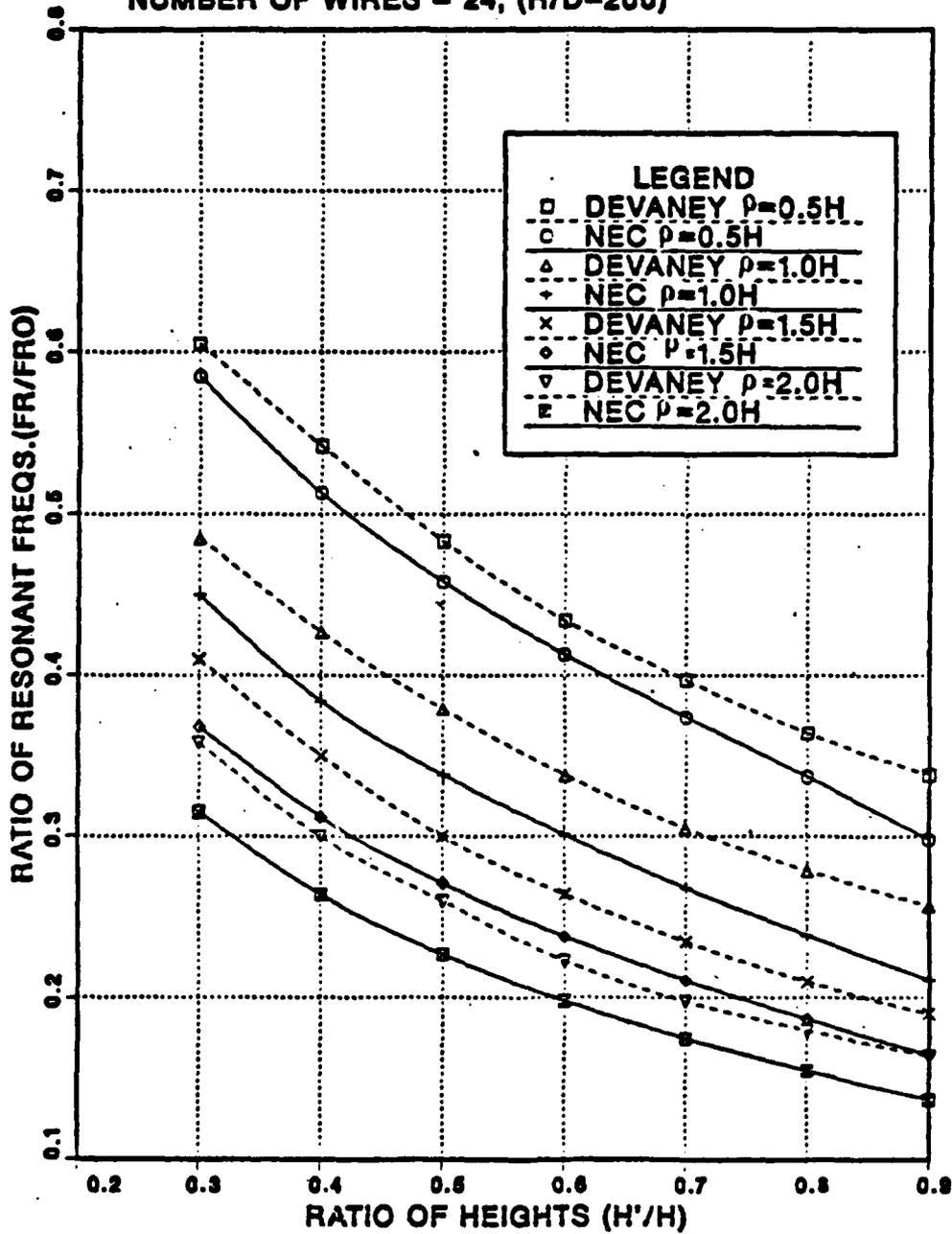
Figure A.9 Normalized Resonant Frequency of Top-Loaded Antenna, the Number of Top-Hat Radials  $N = 24$ .
