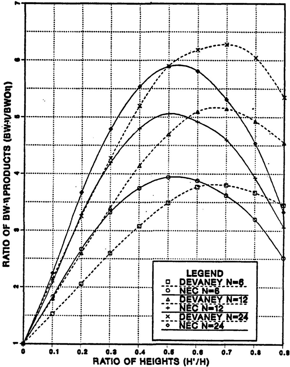
Figure 3.15 Normalized Bandwidth-Efficiency Product of Top-Loaded Antenna,  $\rho = H$ .
