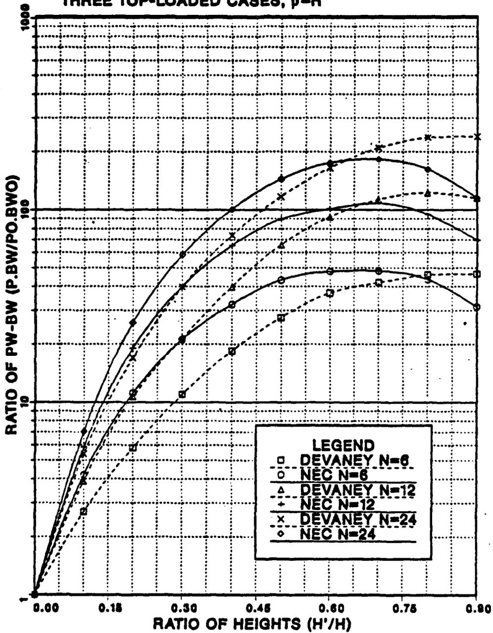
Figure 3.17 Normalized Power-Bandwidth Product of Top-Loaded Antenna,  $\rho = H$ .
