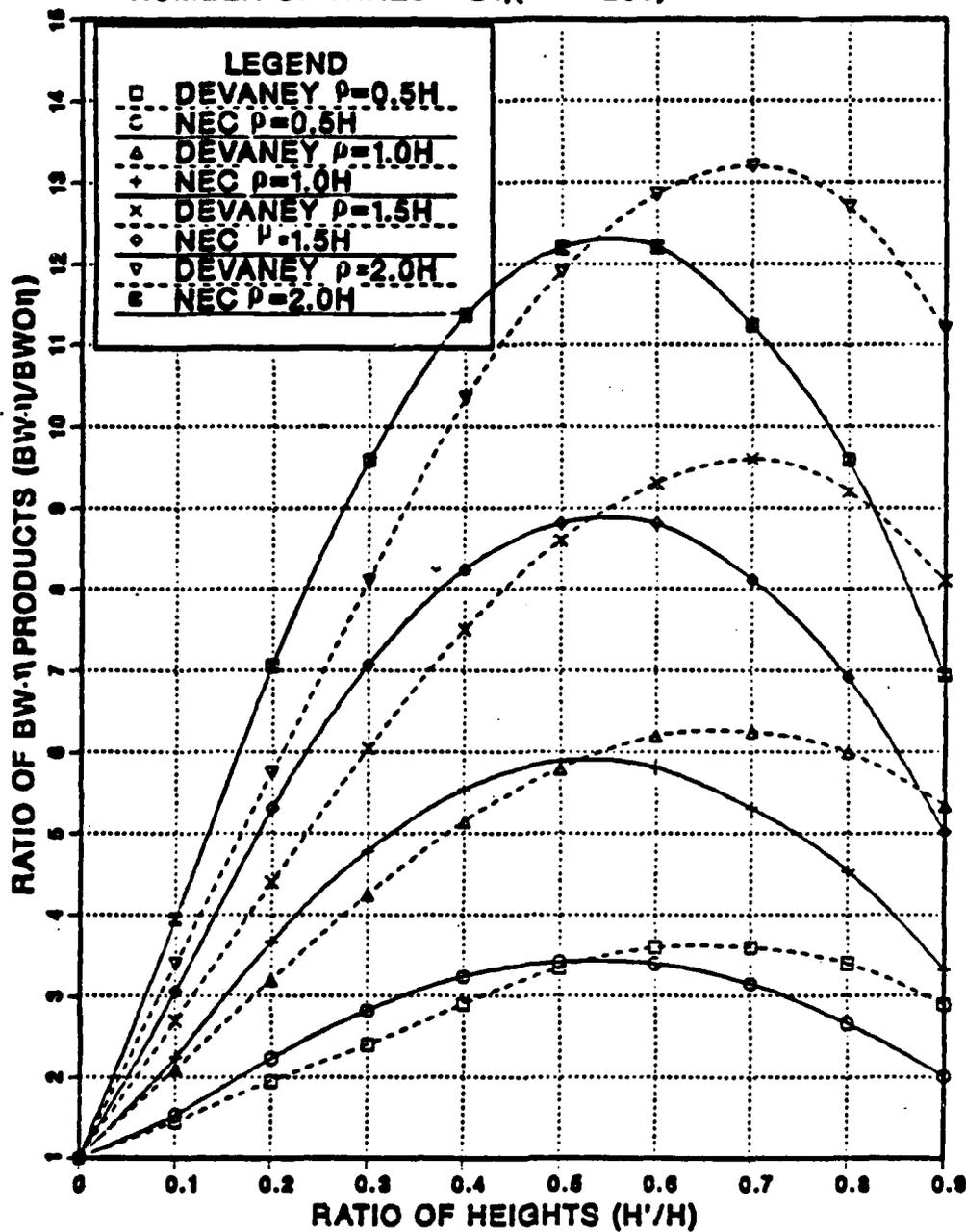
Figure A.12 Normalized Bandwidth-Efficiency Product of Top-Loaded Antenna, the Number of Top-Hat Radials  $N = 24$ .
