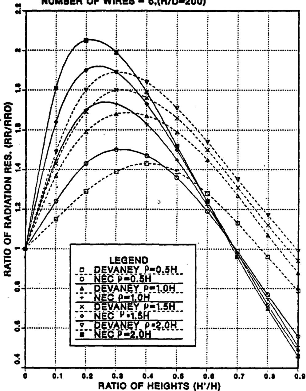
Figure 3.11 Normalized Radiation Resistance of Top-Loaded Antenna, the Number of Top-Flat Radials  $N = 6$ .
