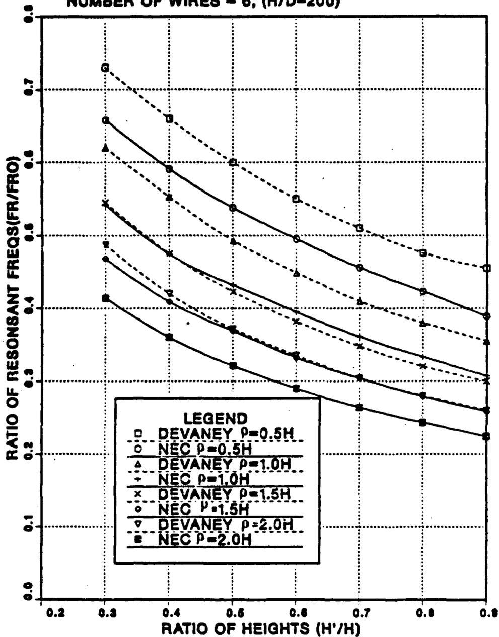
Figure 3.9 Normalized Resonant Frequency of Top-Loaded Antenna, the Number of Top-Hat Radials  $N = 6$ .
