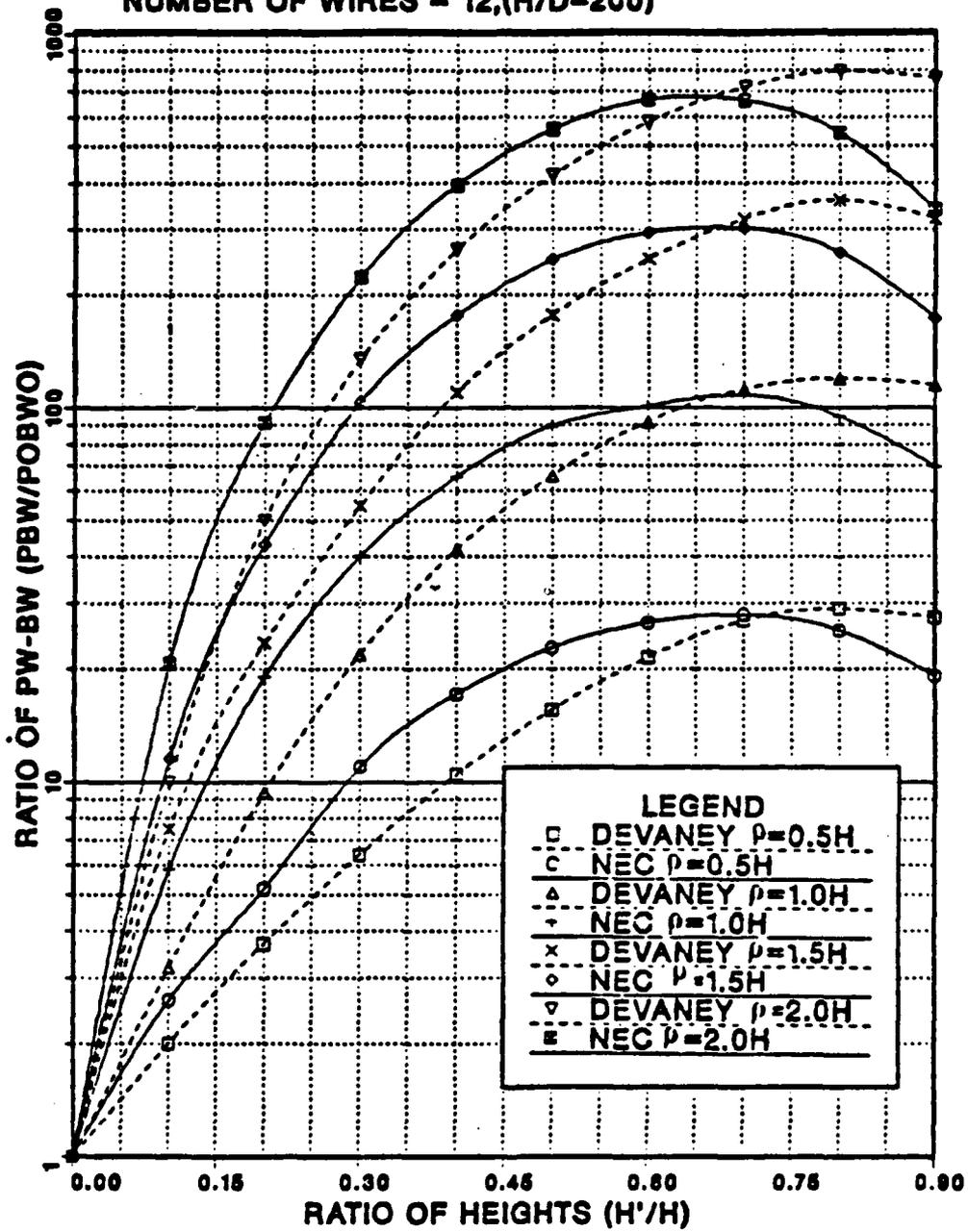
Figure A.7 Normalized Power-Bandwidth Product of Top-Loaded Antenna, the Number of Top-Hat Radials  $N = 12$ .
