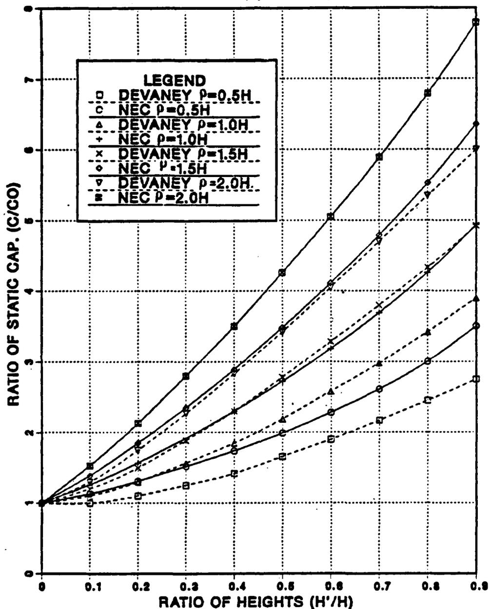
Figure 3.8 Normalized Static Capacitance of Top-Loaded Antenna, the Number of Top-Hat Radials  $N = 6$ .
