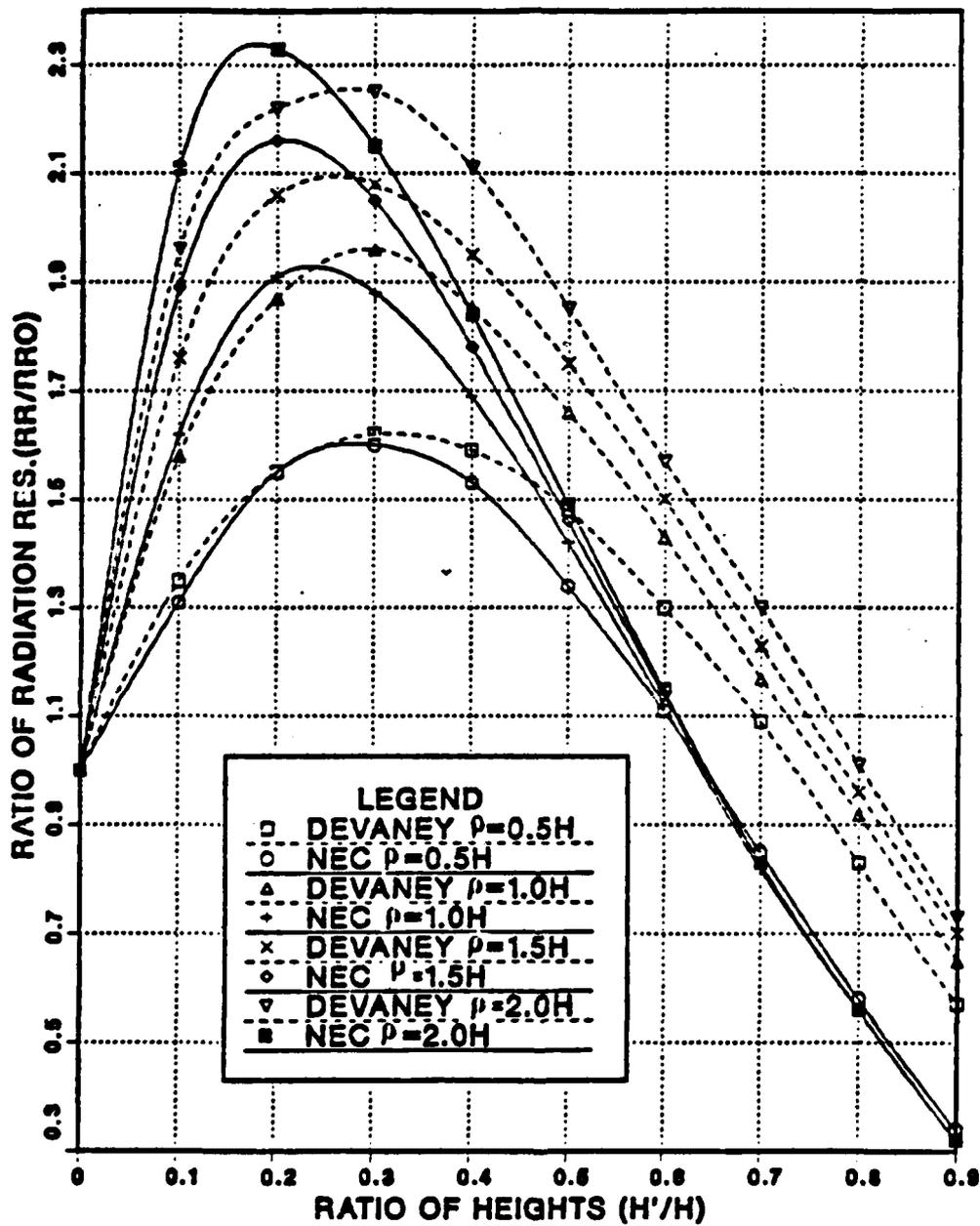
Figure A.11 Normalized Radiation Resistance of Top Loaded Antenna, the Number of Top-Hat Radials  $N = 24$ .
