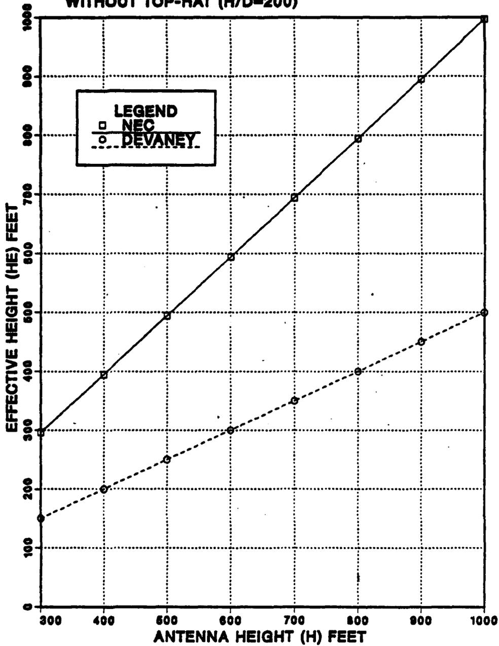
Figure 3.3 Variation of Effective Height of Reference Antenna as a Function of Antenna Height.
