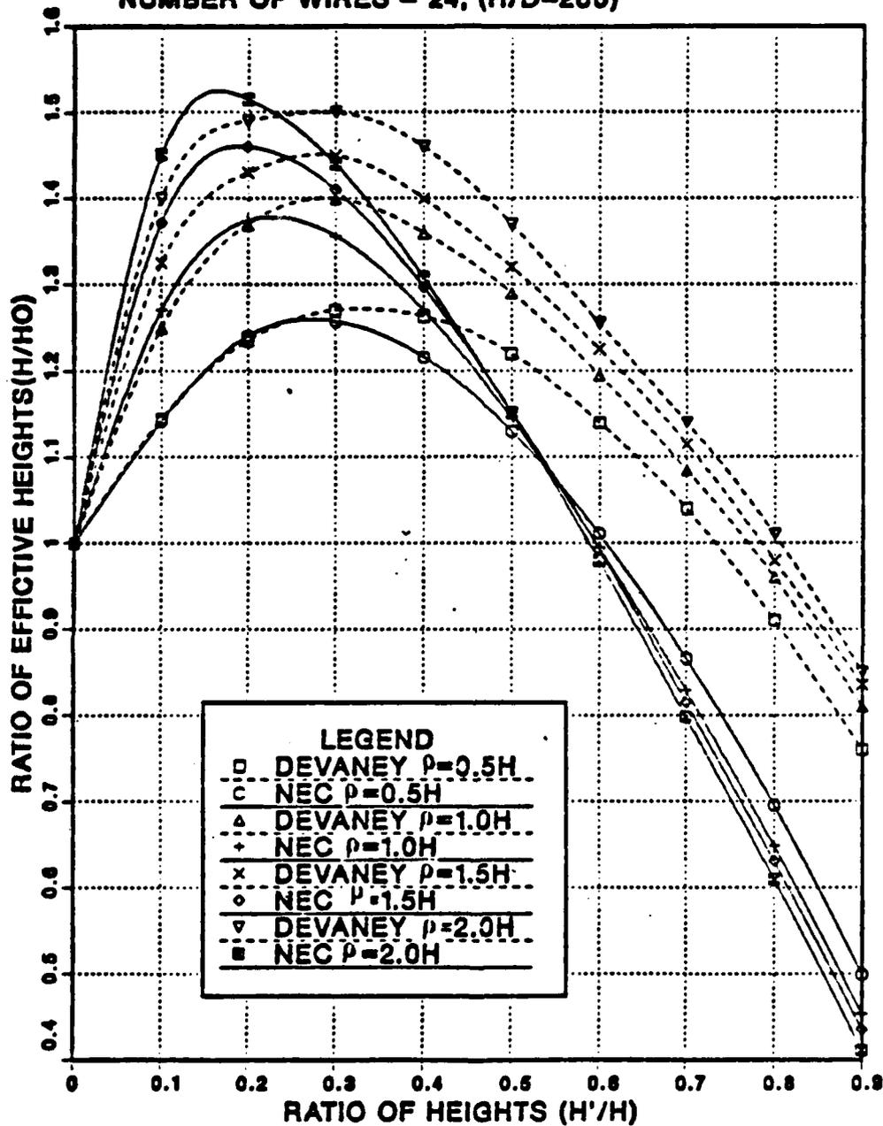
Figure A.10 Normalized Effective Height of Top-Loaded Antenna, the Number of Top-Hat Radials  $N = 24$ .
