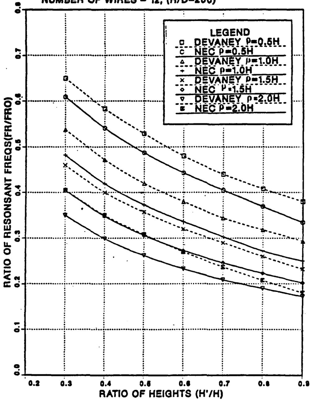
Figure A.2 Normalized Resonant Frequency of Top-Loaded Antenna, the Number of Top-Hat Radials  $N = 12$ .
