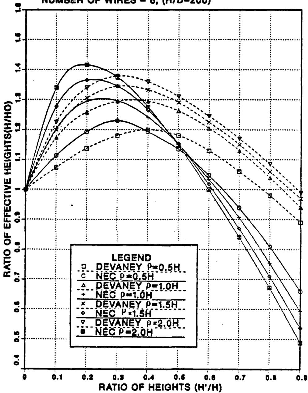
Figure 3.10 Normalized Effective Height of Top-Loaded Antenna, the Number of Top-Hat Radials  $N = 6$ .
