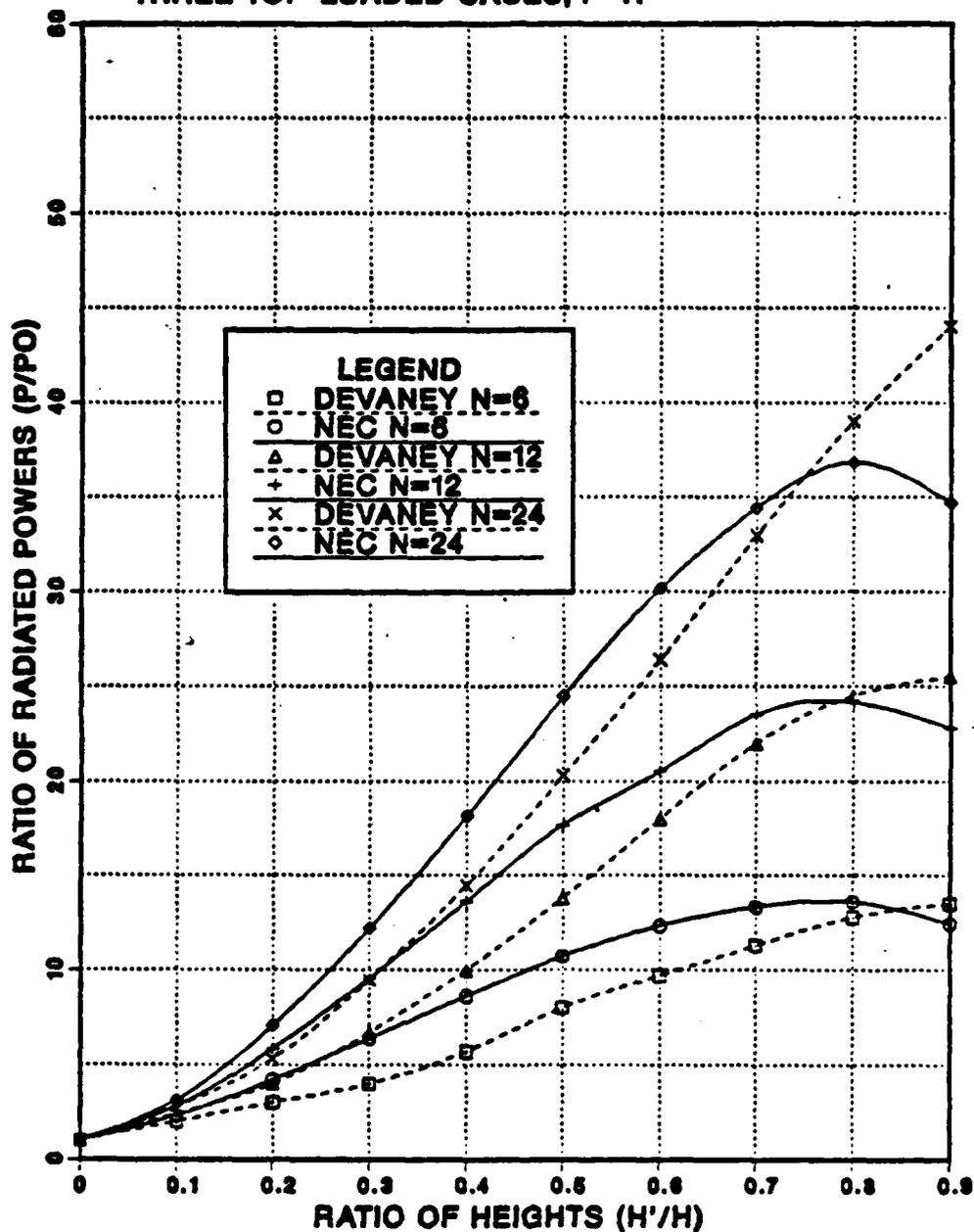
Figure 3.16 Normalized Maximum Radiated-Power of Top-Loaded Antenna,  $\rho = H$ .
