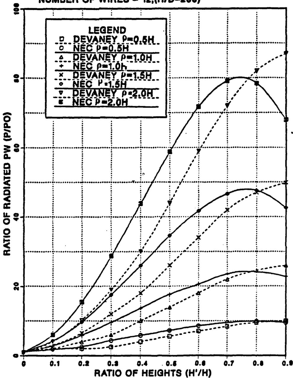
Figure A.6 Normalized Maximum Radiated-Power of Top-Loaded Antenna, the Number of Top-Hat Radials  $N = 12$ .
