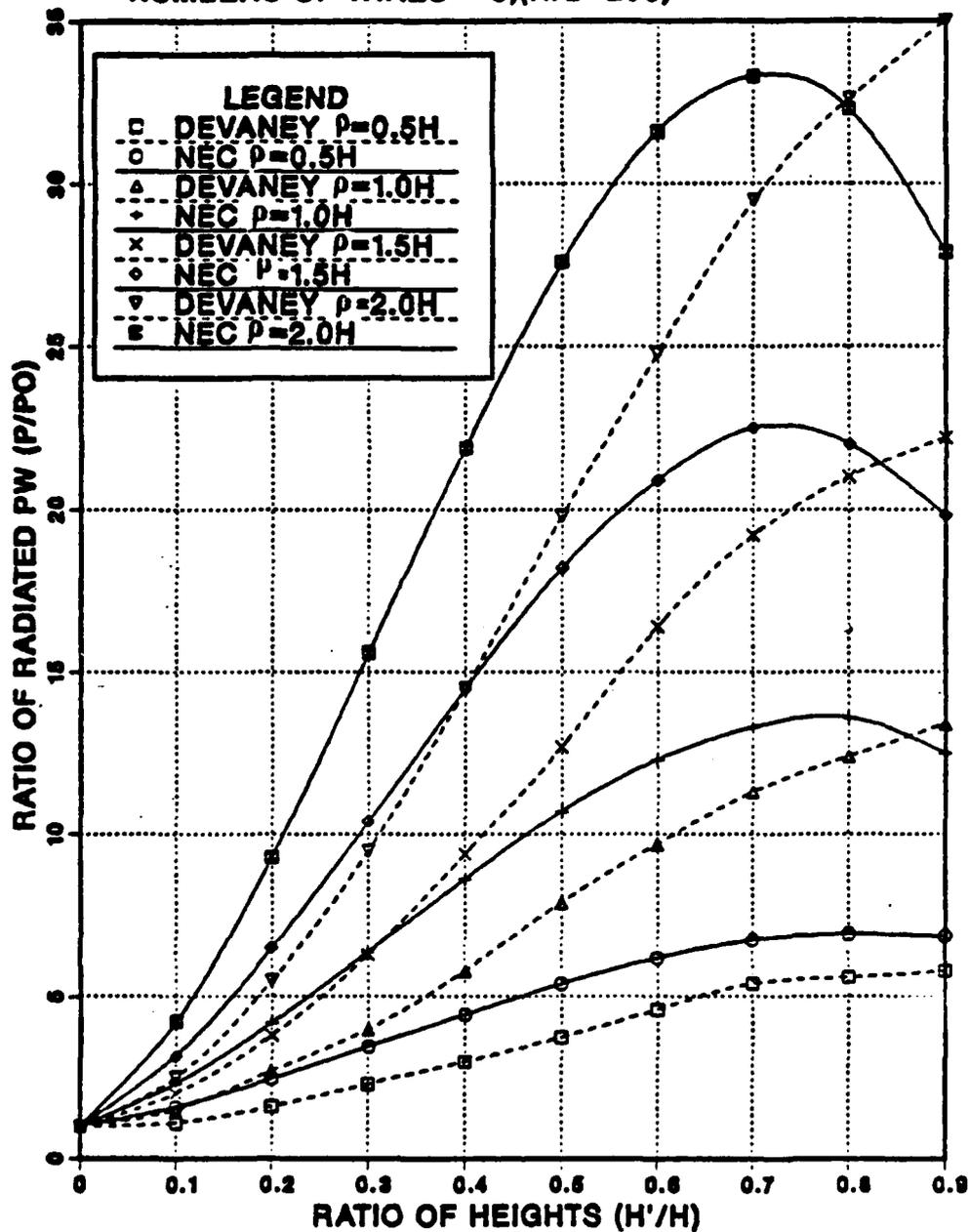
Figure 3.13 Normalized Maximum Radiated-Power of Top-Loaded Antenna, the Number of Top-Hat Radials  $N = 6$ .
