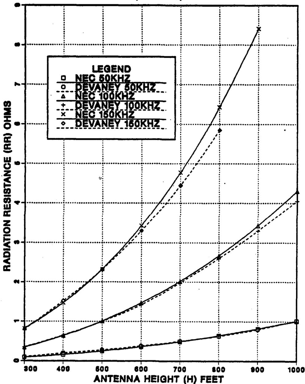
Figure 3.4 Variation of Radiation Resistance of Reference Antenna as a Function of Antenna Height.
