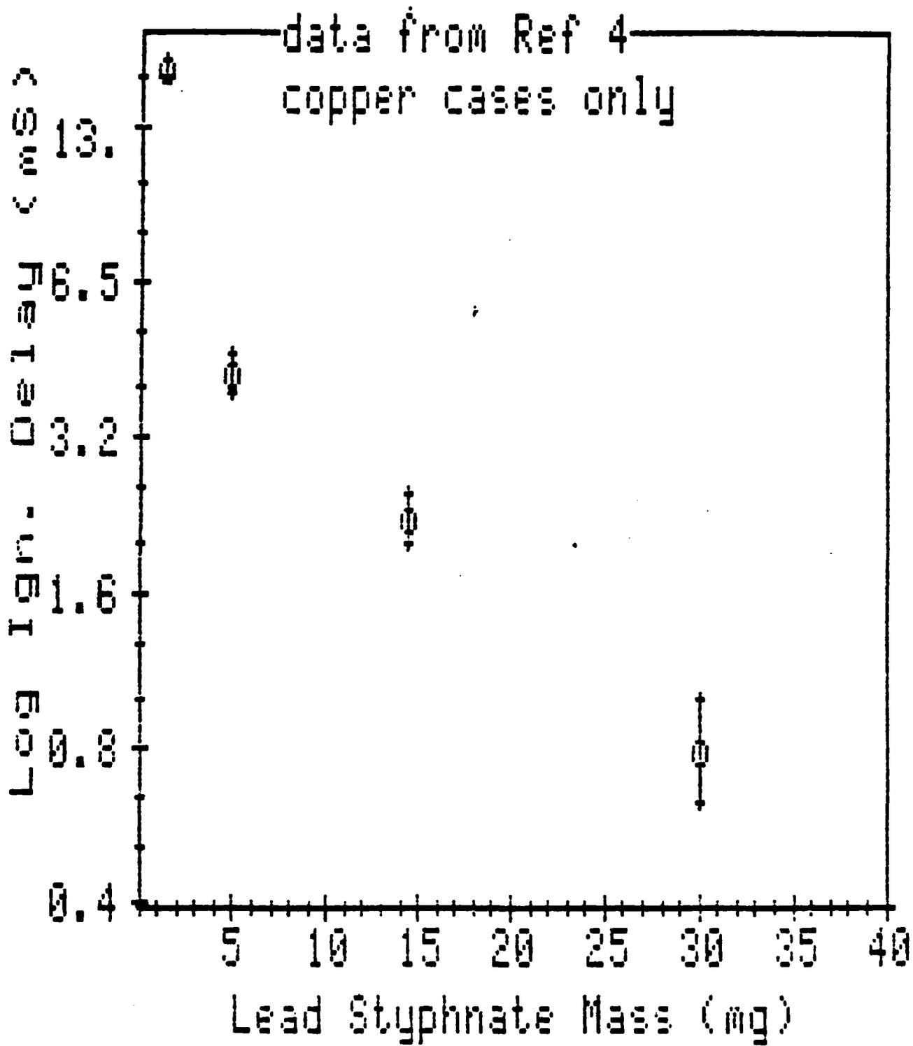
Figure 8. Ignition Delay vs Lead Styphnate Mass.
