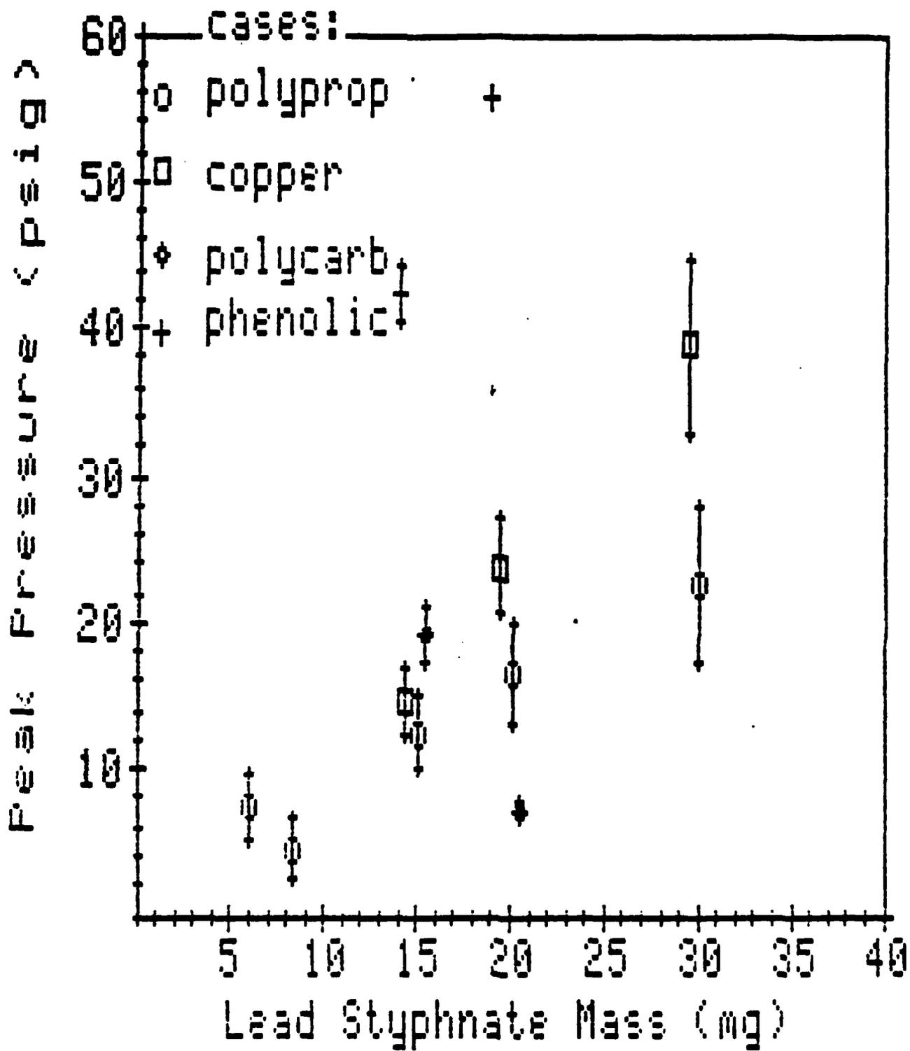
Figure 9. Peak Pressure vs Stage 1 Mass.
