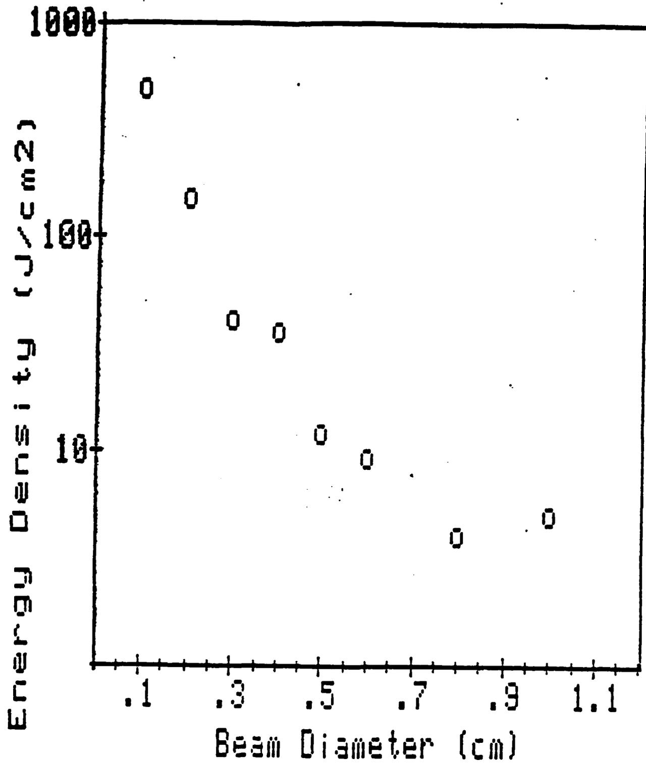
Figure 2. Laser Ignition Boundary of Black Powder.
