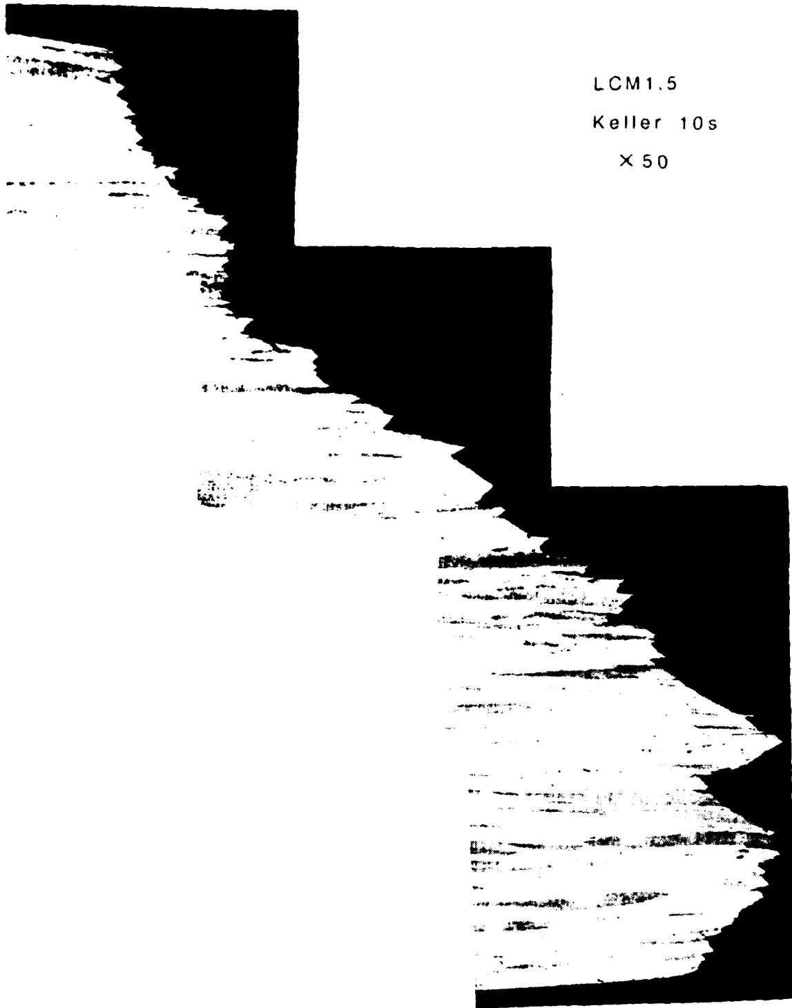
Fig. 10 Sectioned tensile specimen after testing to failure. Alloy LCM1 SHT 30 min. at 550°C, aged 48 hr. at 190°C. (TS plane)
