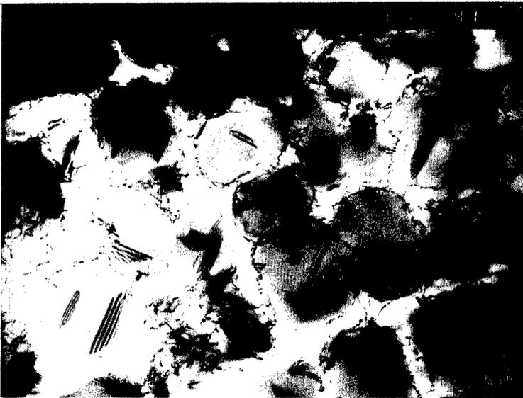
a. High Density of Stack Fault.
