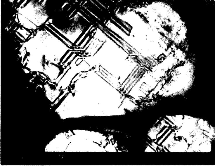
b. Two Sets of Faults in the Precipitate.
