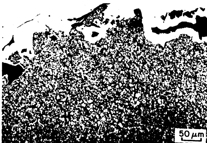
Figure 63. Light micrographs of sub-size charpy impact specimens; Temp = -50 deg.C, Ferritic microstructure.
