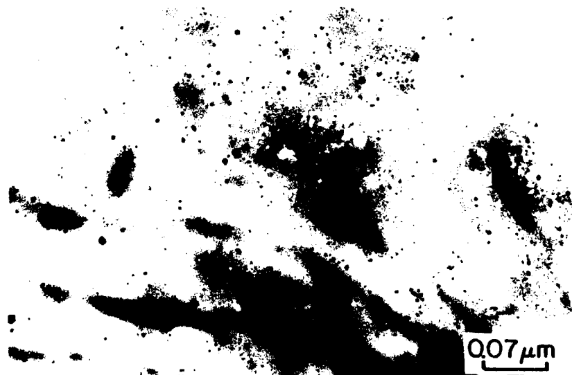
Figure 71. Transmission electron micrograph of thin foil in the diffuse banded region in the HAZ of low heat input weld. (a) Martensitic and ferritic microstructure. (b) Iron carbide precipitation within ferritic grain.
