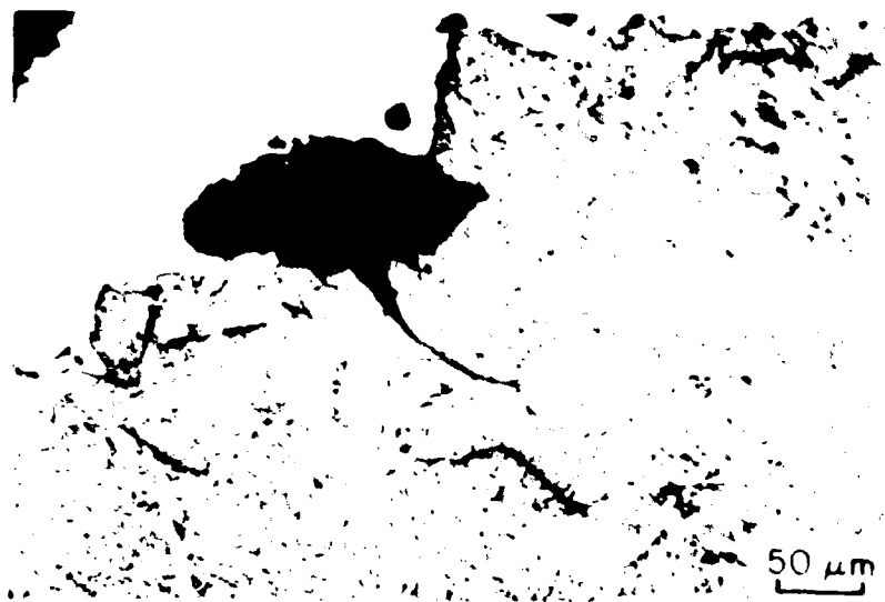
Figure 60. Light micrographs of sub-size Charpy impact specimens; Temp = -50 deg.C, Bainitic/Martensitic microstructure. (a) Profile macrograph of specimen (b) Crack tip profile through Bainitic/Martensitic microstructure
