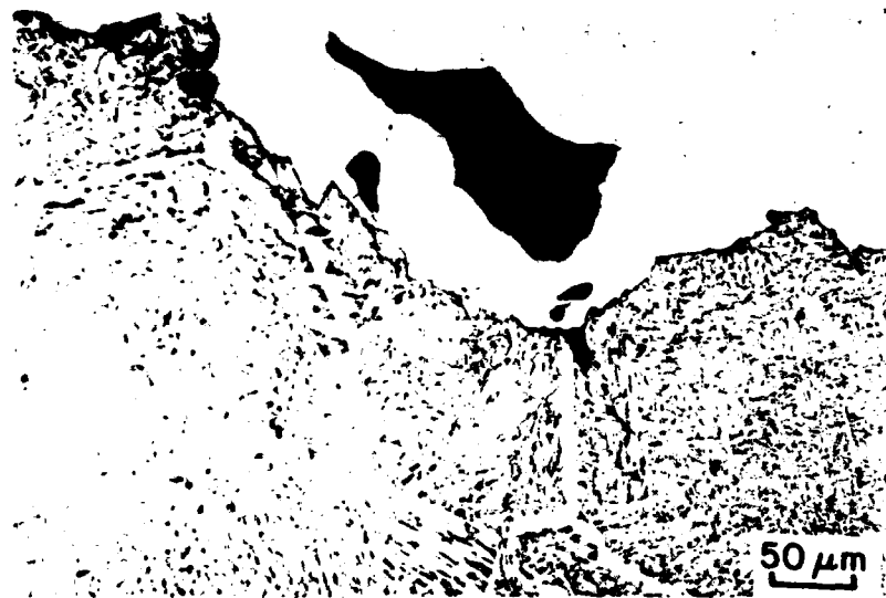
Figure 57. Light micrographs of sub-size Charpy impact specimens; Temp = -50 deg.C, Bainitic microstructure.
