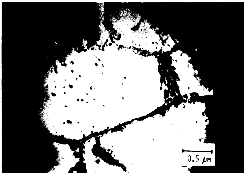
Figure 16. Transmission electron micrograph of 450°C/95 hr heat treated FP( \alpha -alumina)/ZE41A magnesium composite showing the polygonization of the matrix material.
