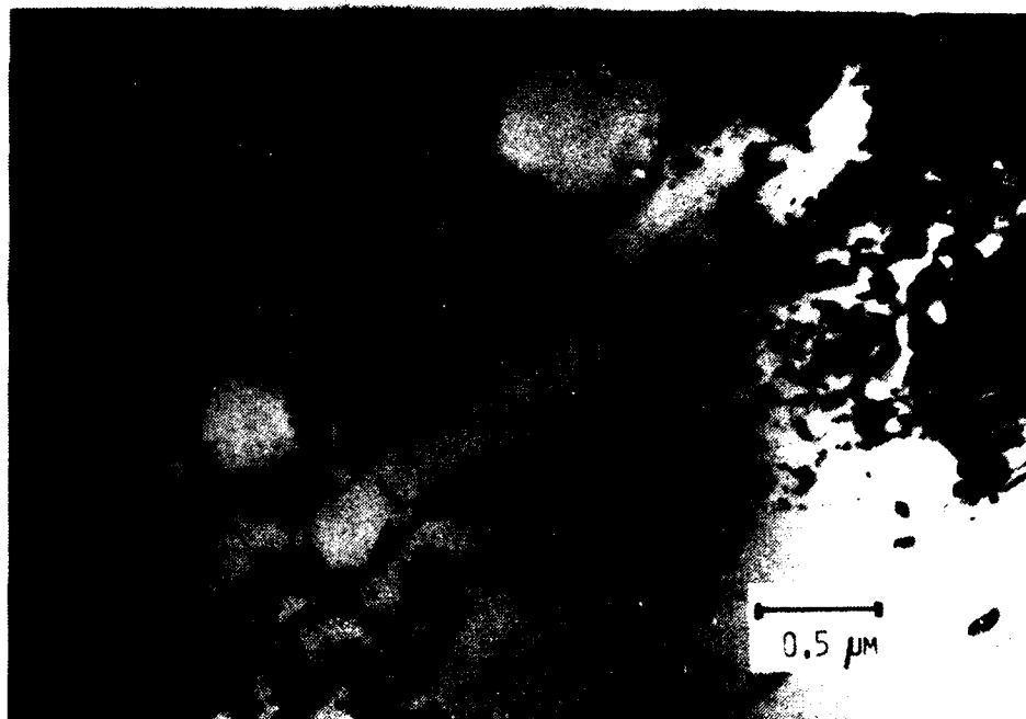
Figure 3. Transmission electron micrograph of as-fabricated FP( \alpha -alumina)/ZE41A Mg revealing (A) the \alpha -alumina fiber, (B) the interfacial reaction zone, and (C) the magnesium matrix.
