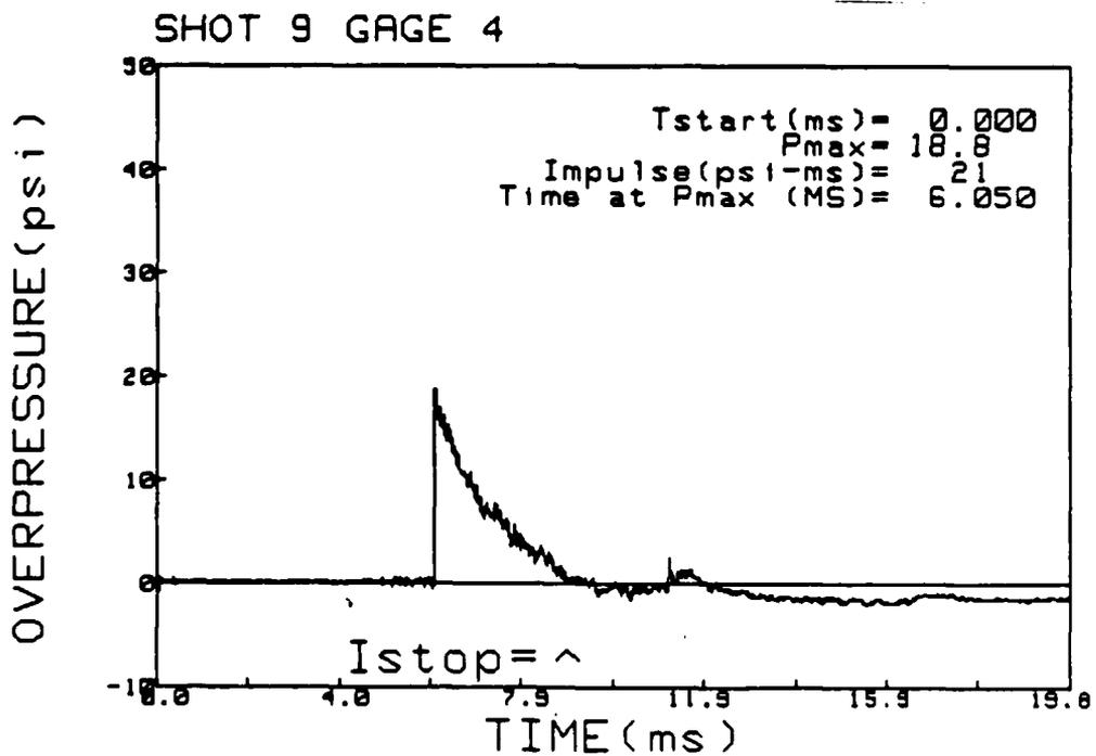
Figure 13b. Pressure-time history for 8 pounds of pentolite with a Pmax of 18.8 psi.
