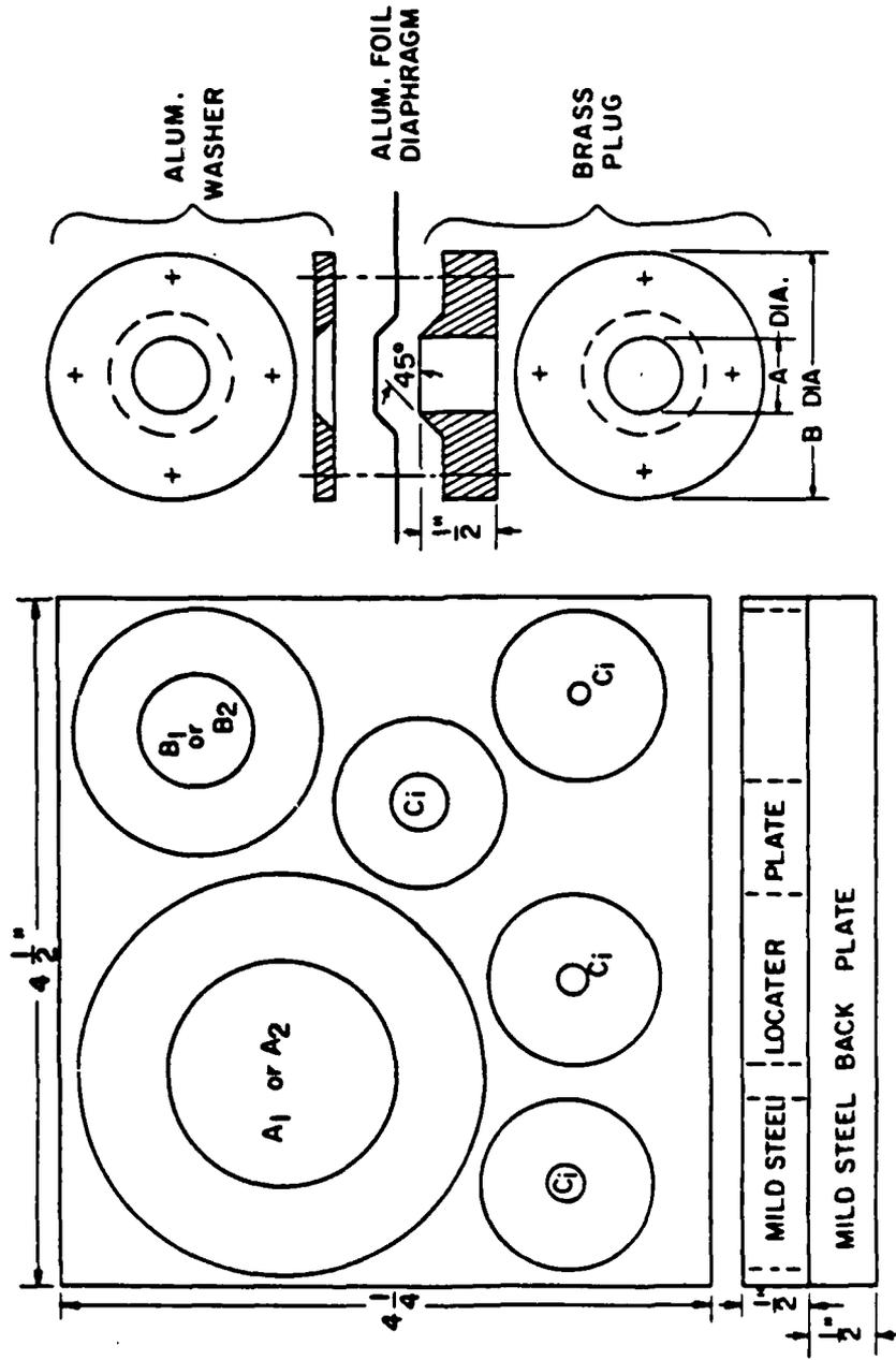
Figure 2. Plan view of the Surface Mounted Discrete Diaphragm Pressure Gage (SMDDPG) and its construction
