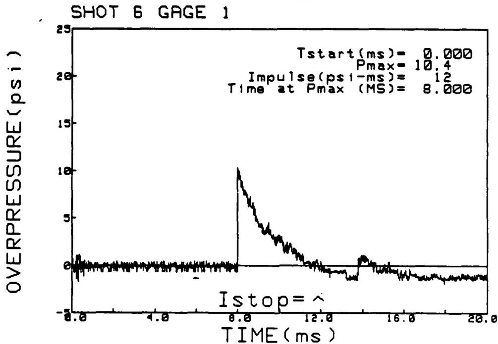
Figure 12b. Pressure-time history for 8 pounds of pentolite with a  $P_{max}$  of 10.4 psi.
