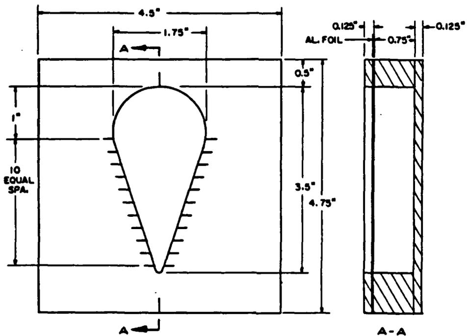
Figure 3a. Plan and end view of the Non-Discrete Diaphragm Pressure Gage (NDDPG)
