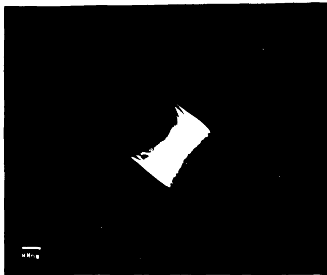
(b) Dark Field Micrograph of Whisker #1 With the (220) Spot Placed on the Optic Axis
