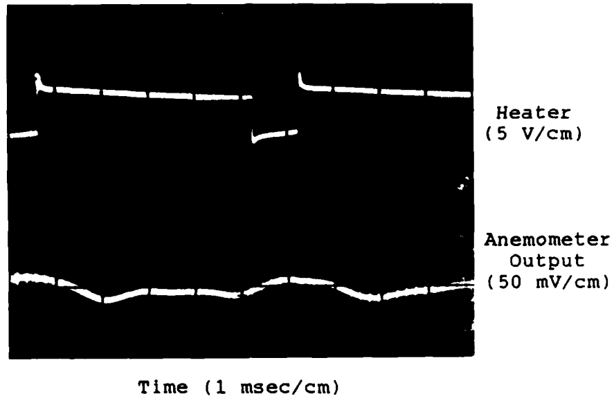
Fig 18. Periodic heating of ribbon, y = 0.06 in, y/\delta = 0.74 . Pulsed heating at 177.5 Hz, ribbon allowed to vibrate.
