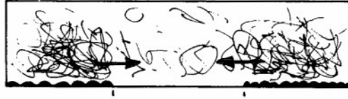
Fig.16 Stress-induced secondary flow in duct with partly-rough wall - secondary flow tends to be down gradient of turbulent intensity.
