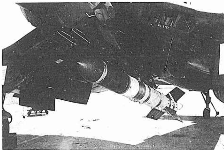
Displacement launcher developed for Tiny Tim (F4U).
