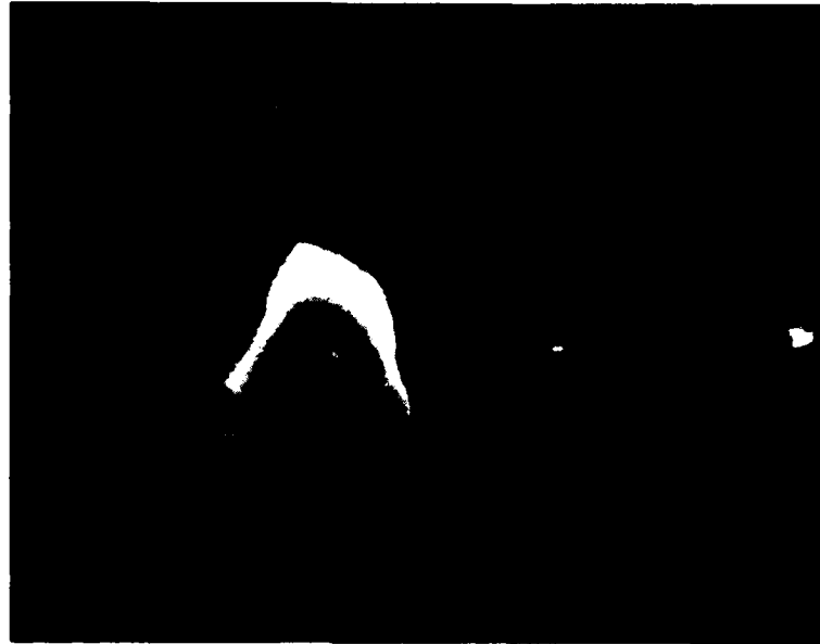
Figure 2-21. 7,500X SEM Photo Of GaAs Particle On ZnSe Surface (Bright Spots Are Result Of Composition Analysis By EDAX).
