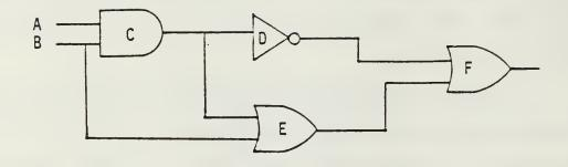
Figure 5. The Four-Element Demonstration Circuit [Ref. 6, p. 43]
