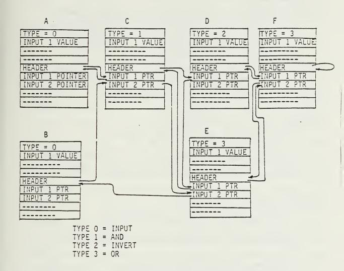
Figure 6. Descriptor Interconnections for the Demonstration Circuit [Ref. 6, p. 43]
