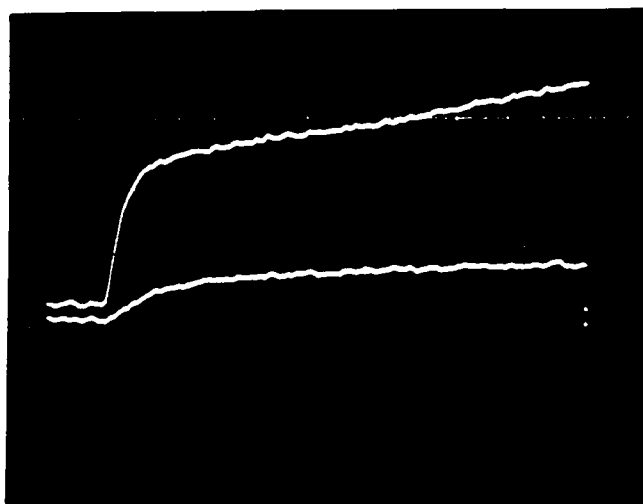
Figure 2A 00^0_1 \rightarrow 00^0_2 P(37) 20 \mu s full scale 50 shots TOP: CO 2 /N 2 O 4/1 mixture 2.5 torr BOTTOM: He/CO 2 /N 2 O 16/4/1 mixture 10.5 torr
