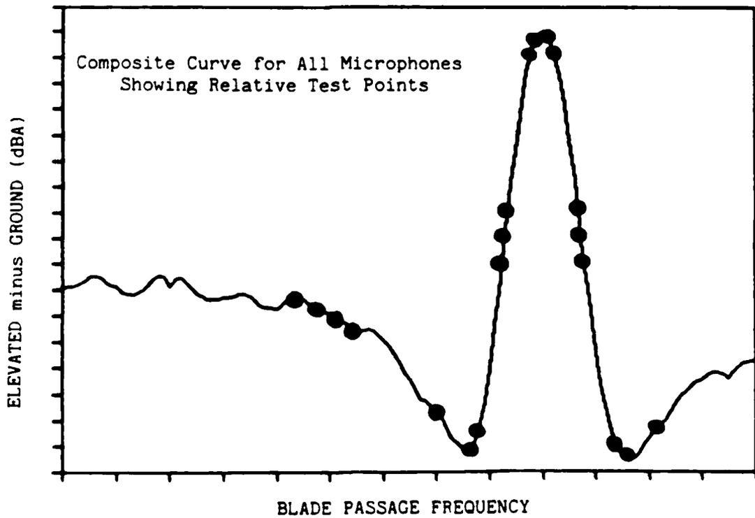
FIGURE 14 DELTA SPL(H) vs. BPF Curves for CARAVAN Test
