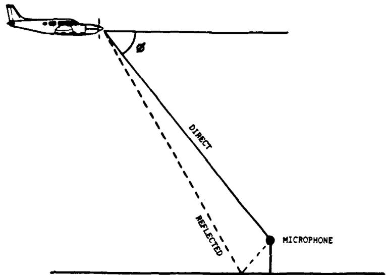
FIGURE 2. Theoretical Ground Interference for a 4 ft. Elevated Microphone
