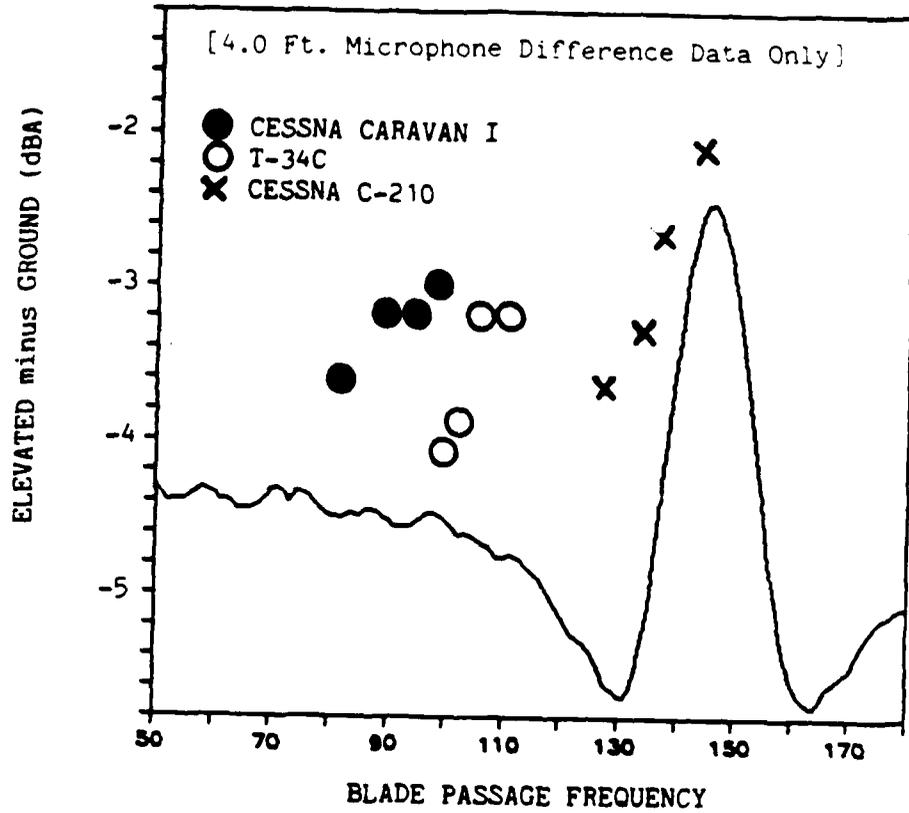
Figure 17 Difference in Noise Levels (elevated minus ground) versus Blade Passage Frequency
