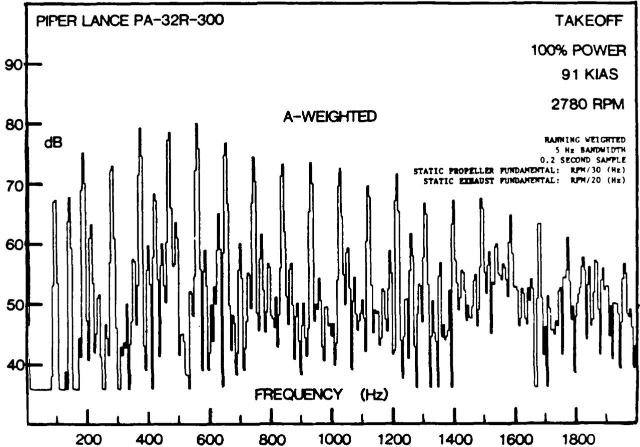
FIGURE 5 Example Spectral Irregularities With an Elevated Microphone
