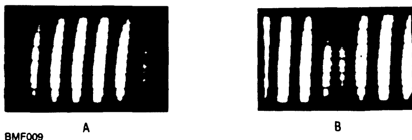
Figure 9. Holograms of Antenna. In A the antennas of the LPA radiated in phase; in B, out of phase.
