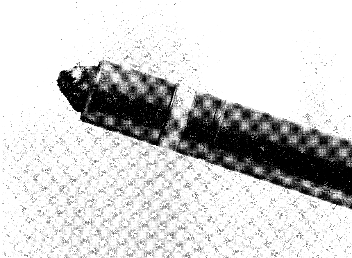
Figure 5-30. Injector Tip with Carbon Deposits
