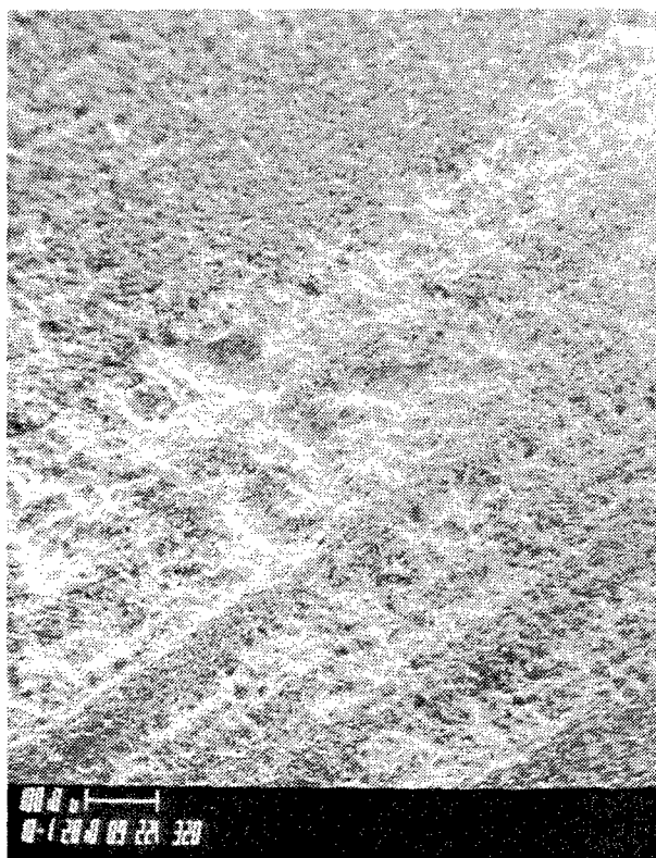
B-5. Magnified View of Wear Track Indicating Brittle Fracture
