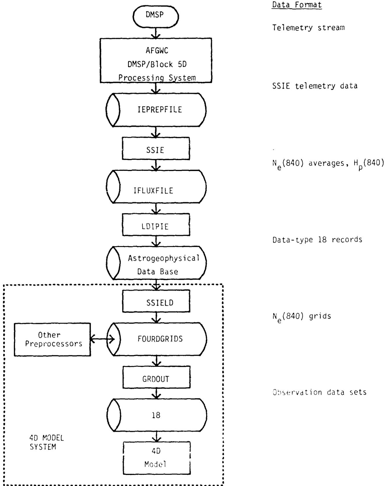
Figure 1. SSIE data processing flow at AFGWC.
