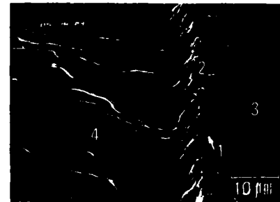
Fig. 1 A partially demineralized fracture surface orthogonal to the joint surface (X2000). Tags (1) are seen in the hybrid (2) which is a porous band. Cured resin is 3 and demineralized dentin is 4.
