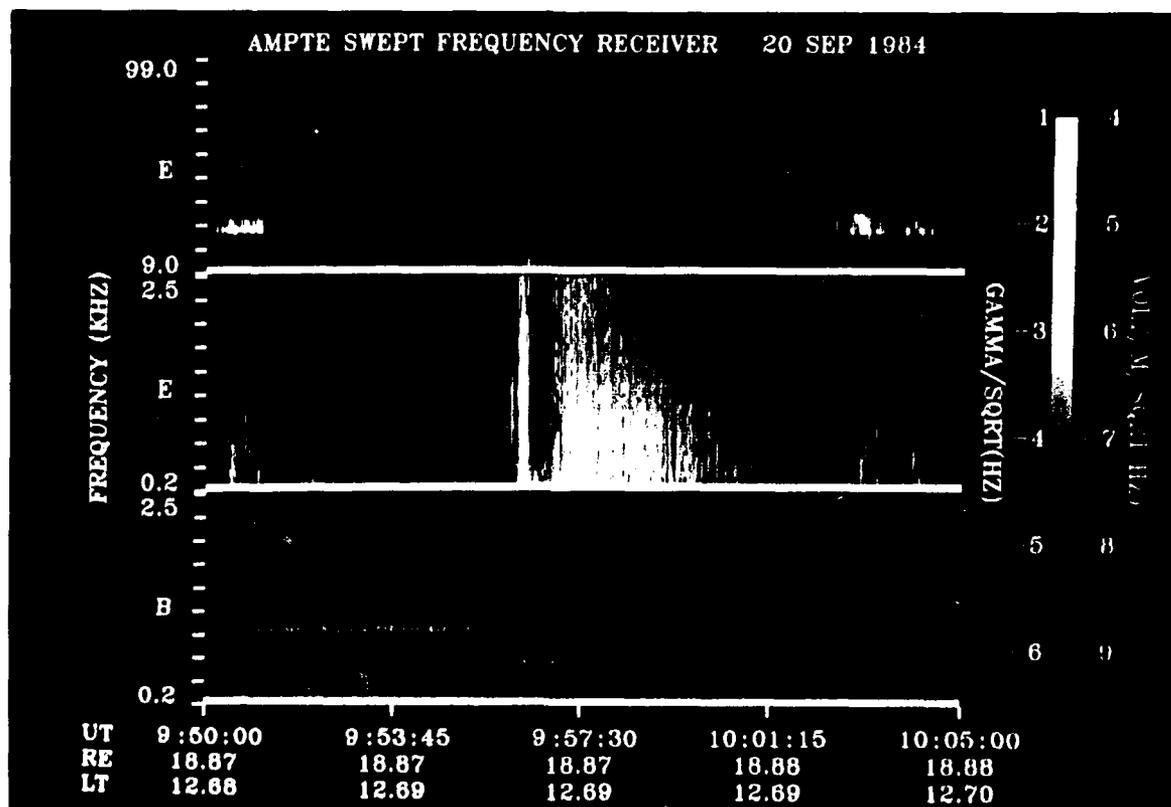
Figure 1. Spectrogram of 15 min of Electric and Magnetic Field Amplitudes over the Frequency Range 200 Hz-100 kHz. The lithium release occurred at 0956:02 UT.
