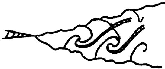
Figure 2. Strained flame sheets (solid lines) and homogeneously mixed zones (cross-hatched) in shear layer.
