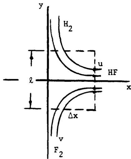
Figure 3. Strained flame control volume.
