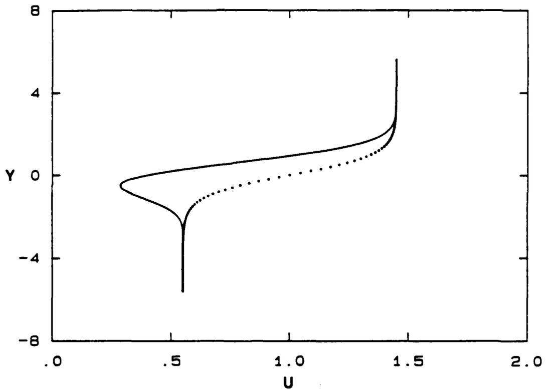
Figure 1a. Mean velocity profile,  $\lambda_0 = 0.45$  ( $U_2/U_1 = 0.38$ ),
