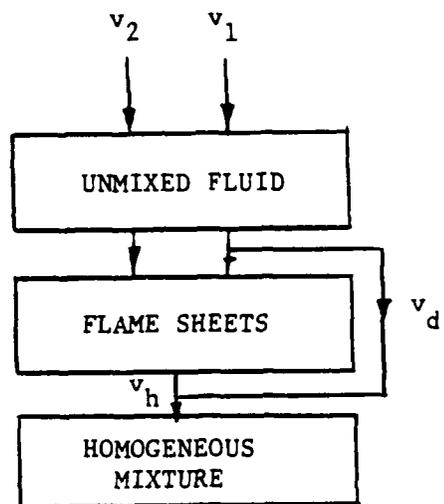
Figure 1. Fluid states in shear layer.
