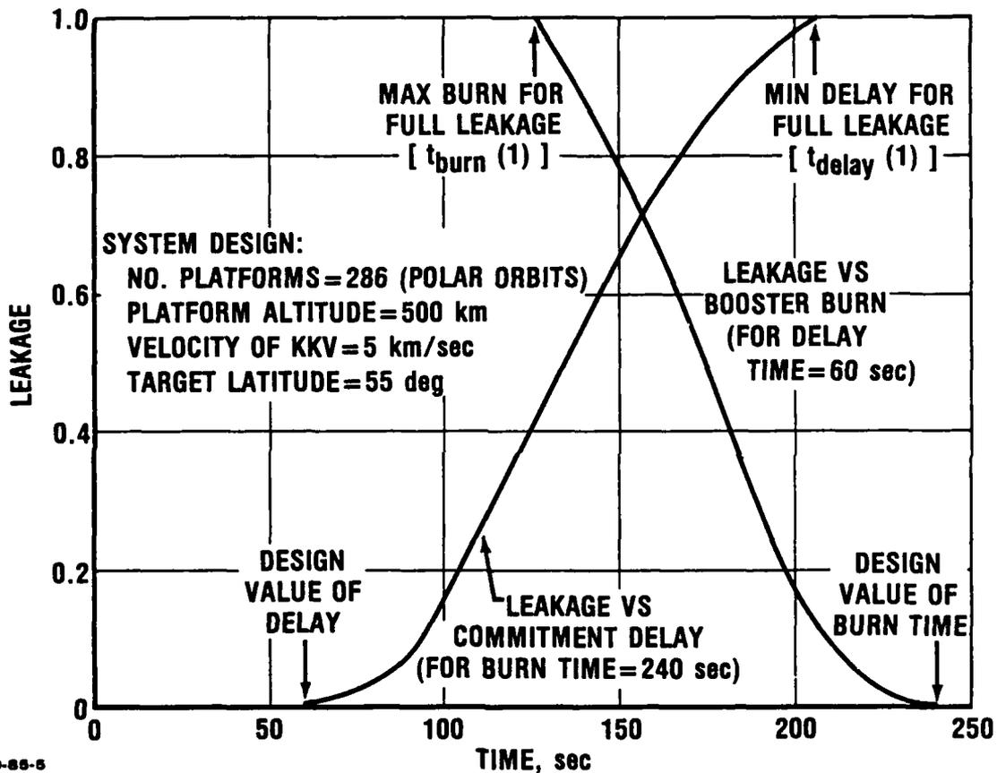
FIGURE 7. Leakage of KEW Boost-Phase-Intercept System Due to Decreased Booster Burn Time and Increased Commitment Delay
