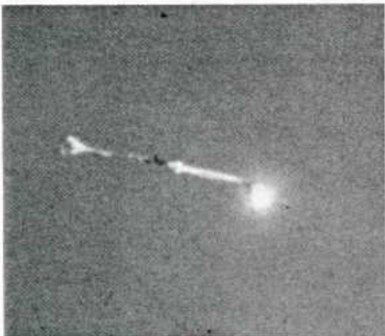
FIGURE 9. Canopy Has Reached Line Stretch and Deployment Bag Has Just Stripped Off. Flashbulb at seat indicates that seat/man separation mechanism has just fired.
