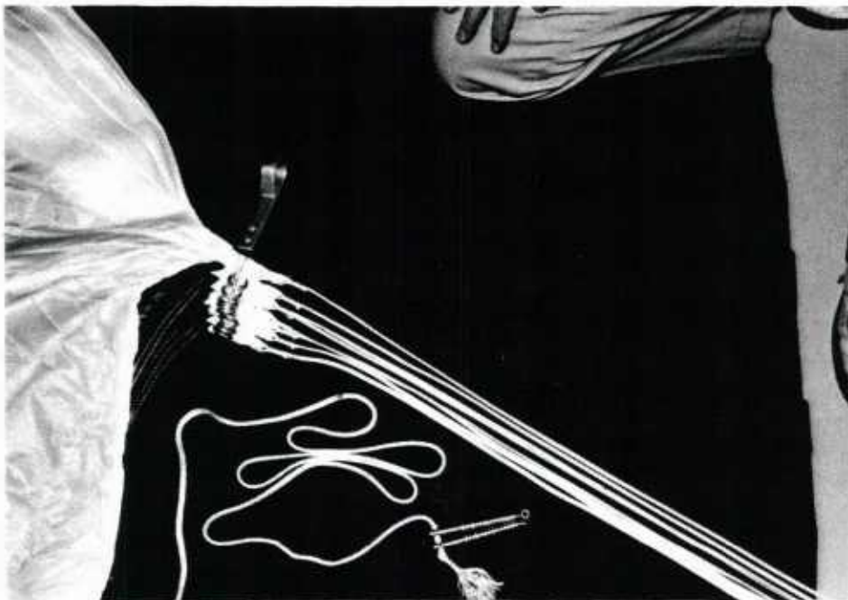
FIGURE A-2. Wire Bodkin Used to Pull Reefing Line Through Rings on the Leading Edge.
