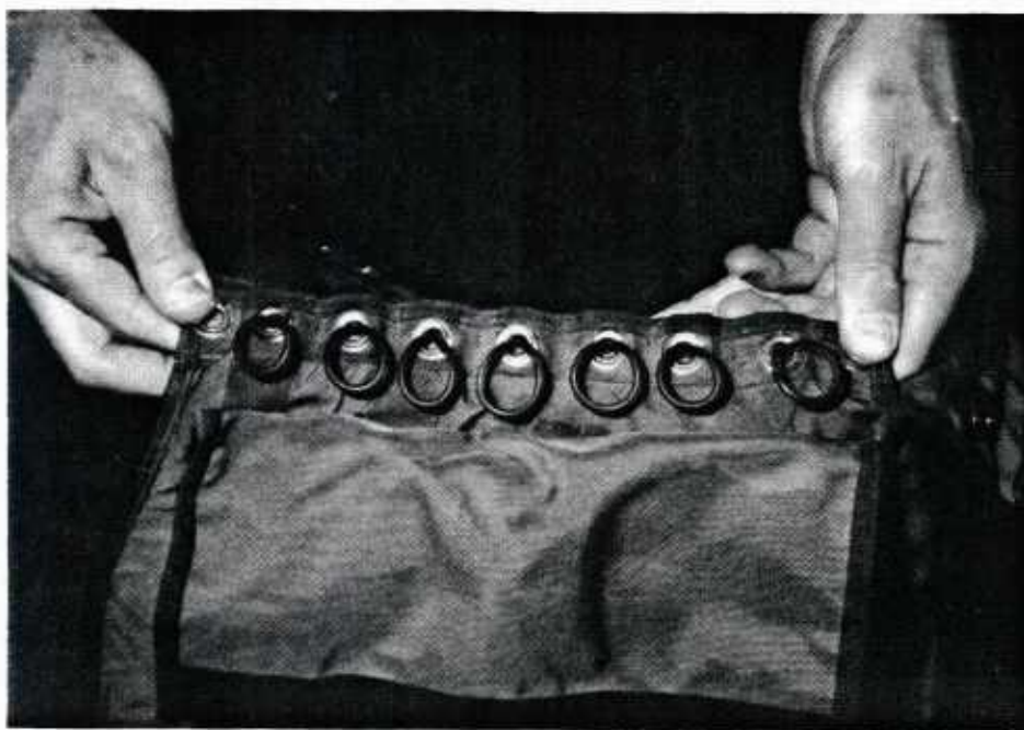
FIGURE 24. Lower Edge of Deployment Bag Showing O-rings Used to Stow Suspension Lines.
