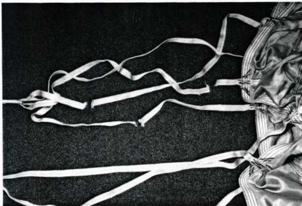
FIGURE 21. Severed Lines on Drogue Canopy.
