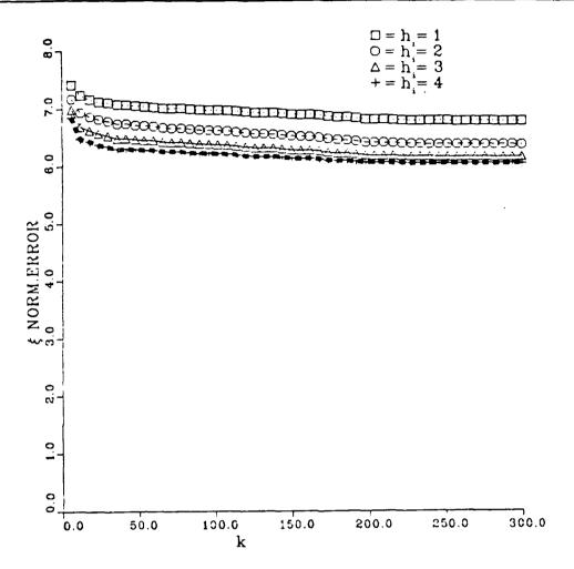
Figure 5-3 Parameter estimation error for four different values of diagonal elements for Venters gain matrix. and p=0.95.
