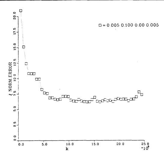
Figure 6-9 Parameter estimation error vs. number of iterations with correlated road noise as the only form of excitation and bias elimination is used.
