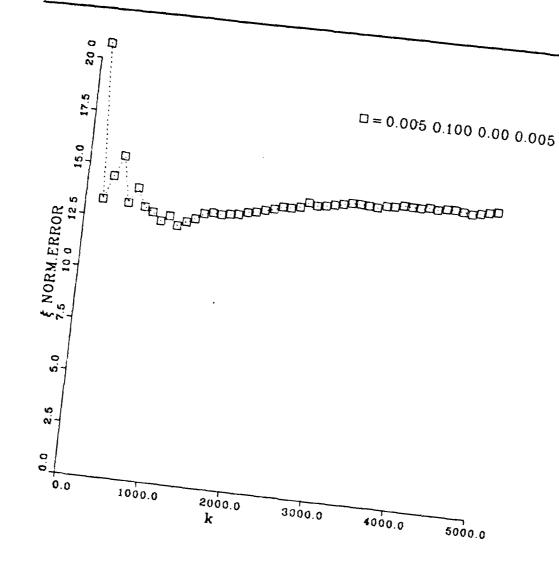
Figure 6-8 Parameter estimation error vs. number of iterations with correlated road noise as the only form of excitation. Initial conditions,  $\sigma=0.0$ Road noise,  $\sigma=0.1$ State measurement noise,  $\sigma=0.0$ State derivative measurement noise,  $\sigma=0.005$
