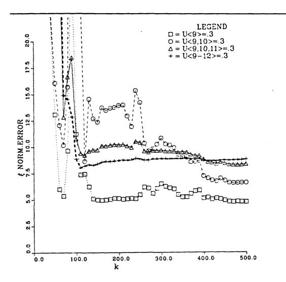
Figure 6-5 Parameter estimation error when system is excited with input pulses of various durations. Pulse duration shown in legend. Initial conditions,  $\sigma=0.01$
