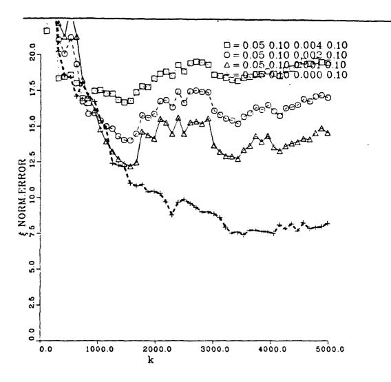
Figure 6-6 Parameter estimation error when various levels of measurement noise are added to the state vector.
