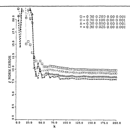
Figure 6-7 Parameter estimation error vs. number of iterations for four different values of road noise, holding initial conditions constant, for two independent noise inputs.
