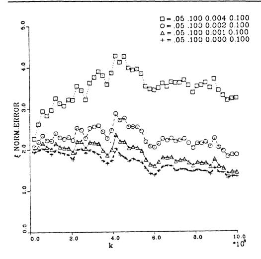
Figure 4-5 Parameter estimation vs. number of iterations with road noise as excitation and various level of state measurement noise. Initial conditions,  $\sigma=0.05$ Road noise,  $\sigma=0.1$
