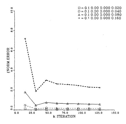
Figure 3-6 Parameter estimation error vs. number of iterations when four different levels of state derivative measurement noise are applied. Initial conditions,  $\sigma=0.1$
