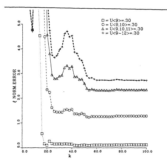
Figure 4-4 Parameter estimation error for various input pulse durations shown in the legend. Initial conditions,  $\sigma=0.01$  Road noise,  $\sigma=0.001$  State measurement noise,  $\sigma=0.0$  State derivative measurement noise,  $\sigma=0.01$ .
