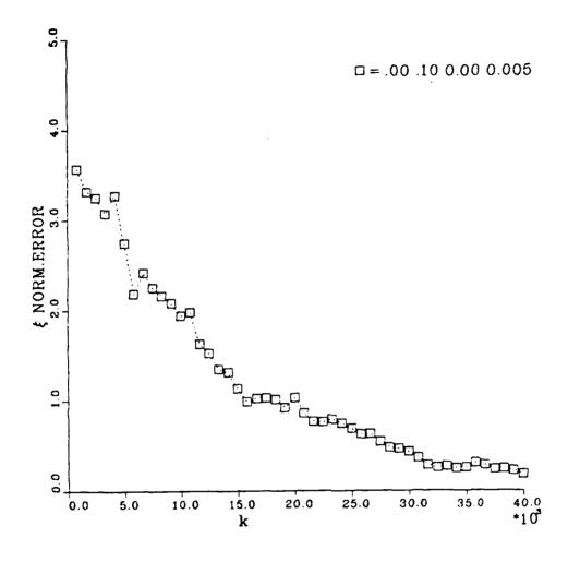
Figure 4-2 Parameter estimation vs. number of iterations with road noise as the only system excitation.
