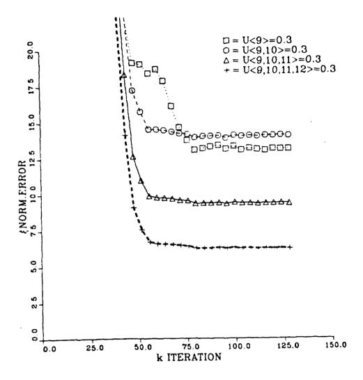
Figure 3-4 Parameter estimation error when pulses of four different widths are used to excite the system. Initial conditions,  $\sigma=0.01$ Road noise,  $\sigma=0.001$ State measurement noise,  $\sigma=0.0$ State derivative measurement noise,  $\sigma=0.0$
