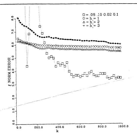
Figure 5-2 Parameter estimation error for Lyapunov gain matrix and three different values of diagonal elements for Venters gain matrix.
