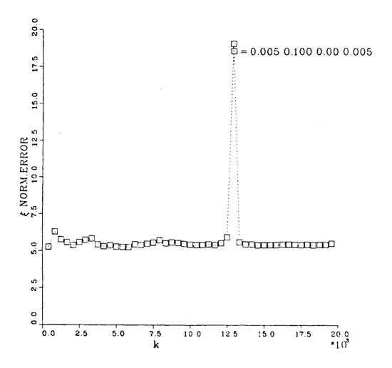
Figure 6-3 Parameter estimation error vs. number of iterations with road noise as the only system excitation. Initial conditions,  $\sigma=0.0$ Road noise,  $\sigma=0.1$ State measurement noise,  $\sigma=0.0$ State derivative measurement noise,  $\sigma=0.005$
