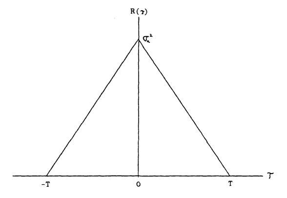
Figure 4-7 Autocorrelation function for discrete road noise with T =0.05
