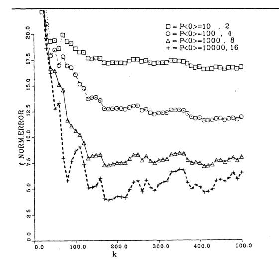
Figure 6-2 Parameter estimation error vs. number of iterations for four different initializations of the covariance matrix. Initial conditions,  $\sigma=0.1$
