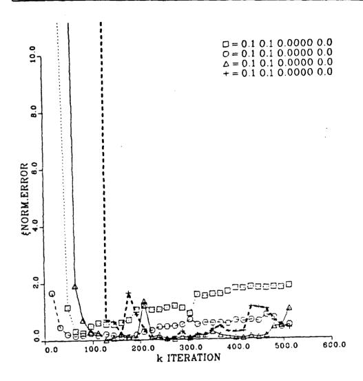
Figure 3-2 Parameter estimation error vs. number of iterations for four different ensembles of road noise.
