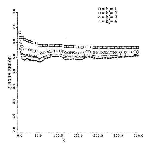
Figure 5-4 Parameter estimation error for four different values of diagonal elements for Venters gain matrix. and the use of a forgetting factor. Initial conditions,  $\sigma=0.08$ Road noise,  $\sigma=0.1$ State measurement noise,  $\sigma=0.02$ State derivative measurement noise,  $\sigma=0.1$
