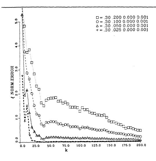
Figure 4-3 Parameter estimation vs. number of iterations with initial conditions and various levels of road noise.
