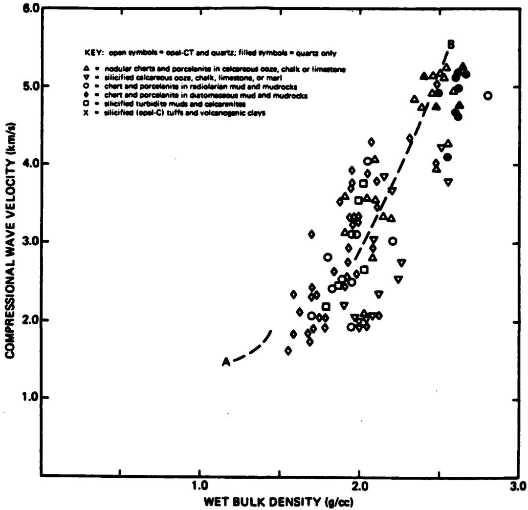
Figure 8. Relation of wet bulk density to compressional wave velocity. From Pisciotto (1981).
