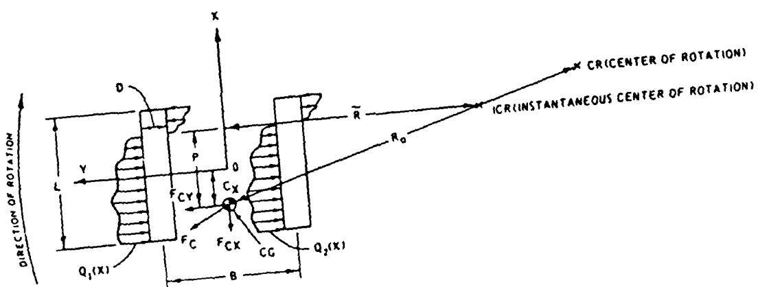
Figure 2.5. Geometry and boundary conditions of the terrain-vehicle model.
