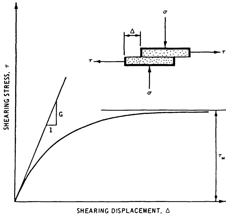
Figure 2.3. Proposed shear stress/deformation relation during shearing process.
