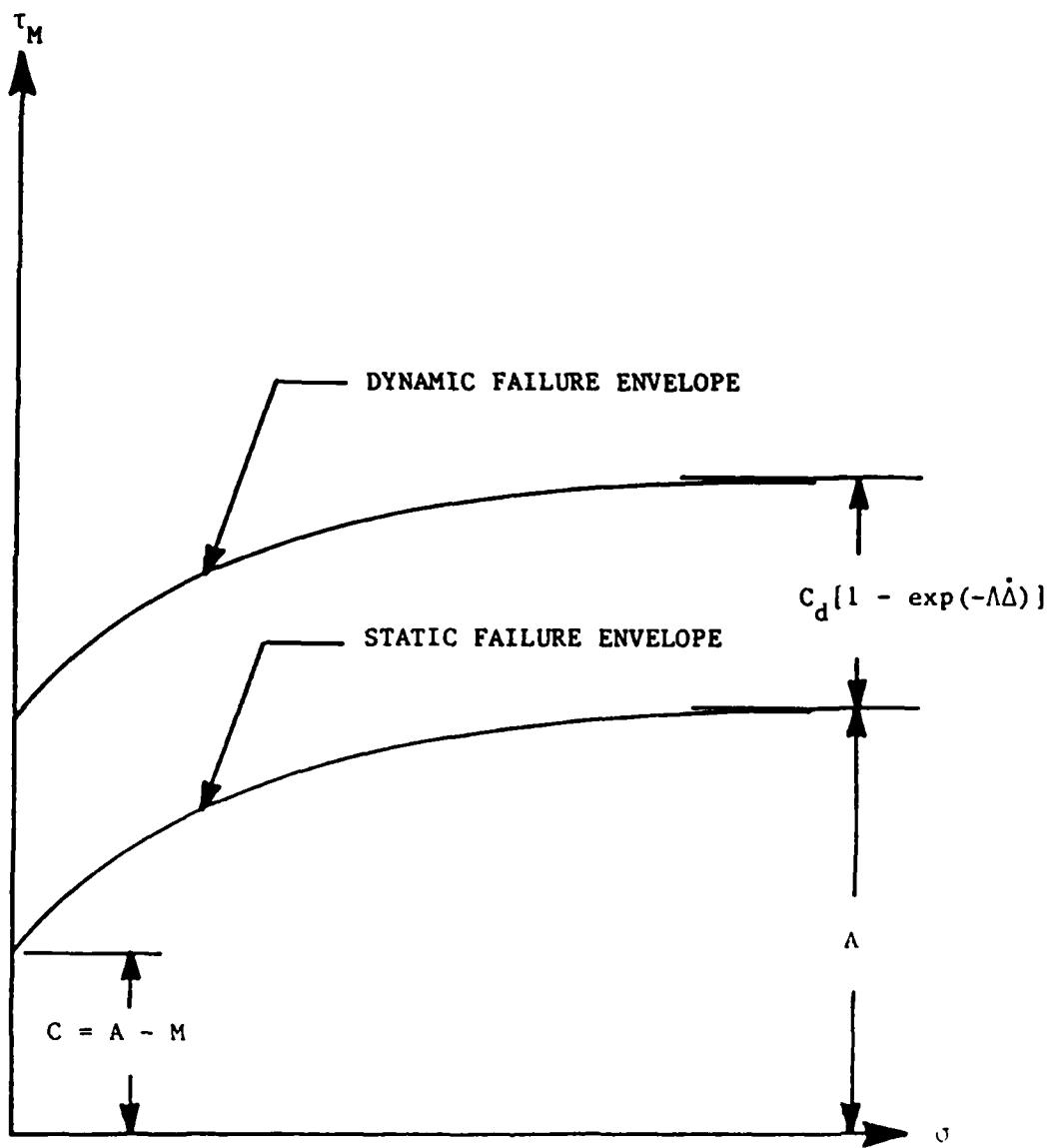
Figure 2.1. Nonlinear shear failure envelope for soil.
