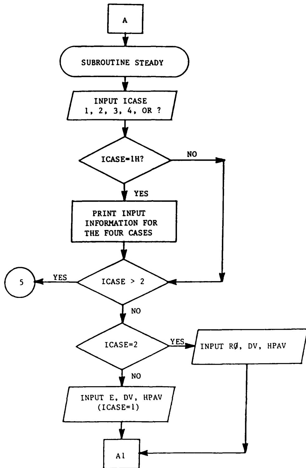
Figure 3.2. Flowchart for subroutine STEADY (Sheet 1 of 4).
