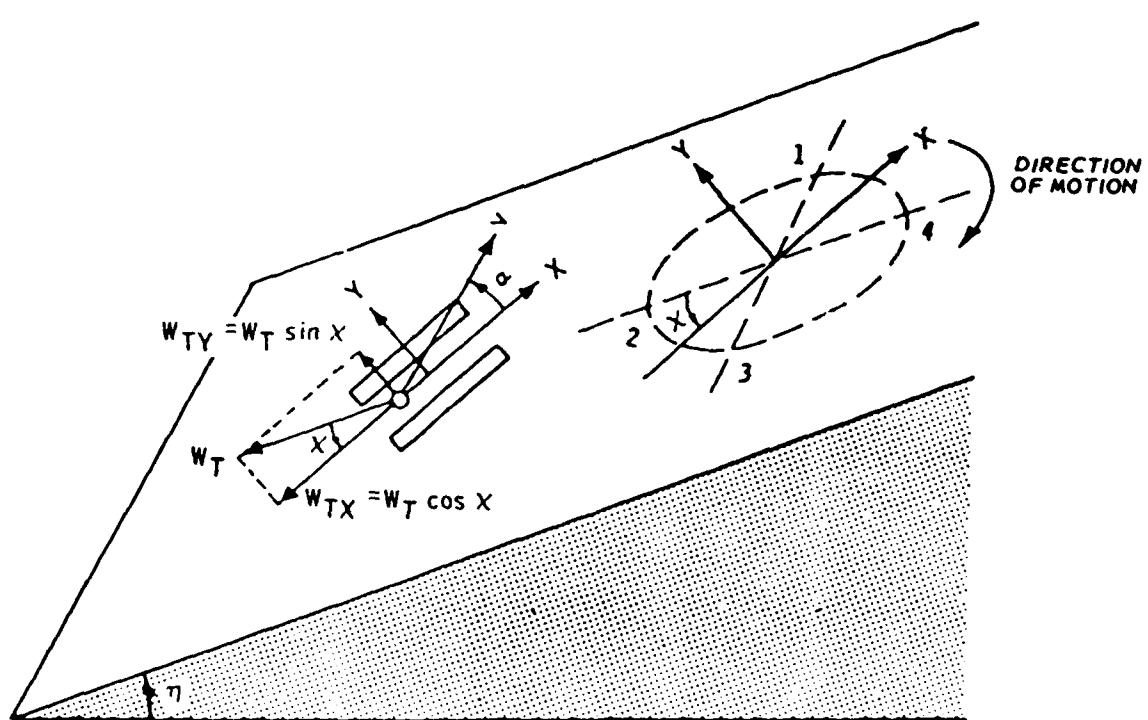
Figure 2.12. Effect of sloping terrain on transient motion.
