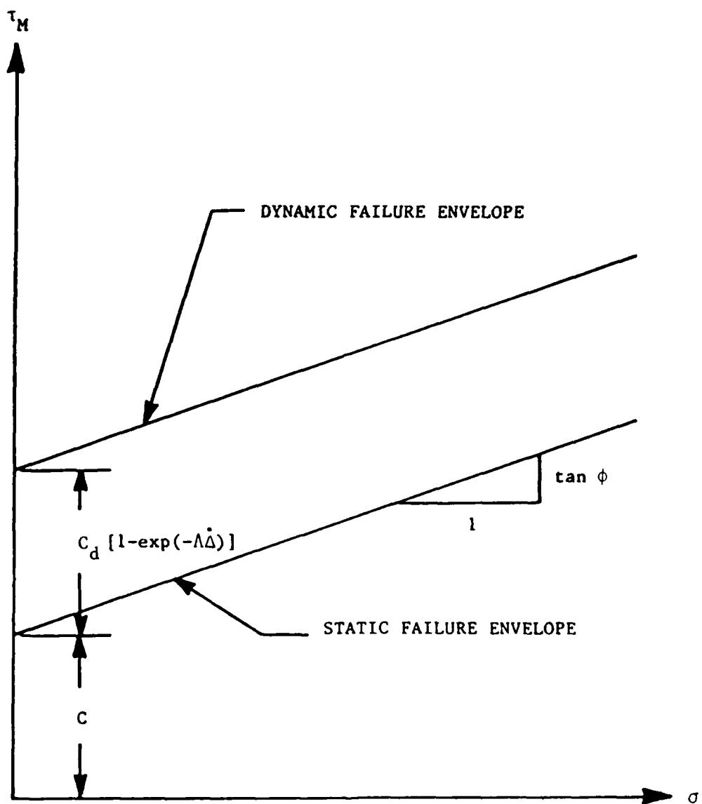
Figure 2.2. Linear shear failure envelope for soil.
