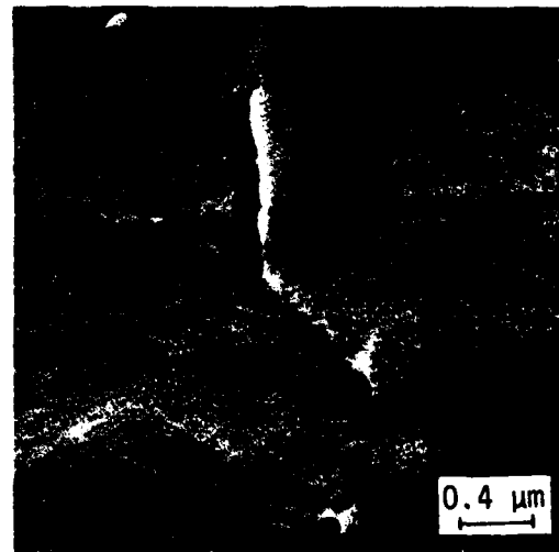
(c) Formation of axial grain boundary microcrack via cavity coalescence.
